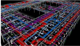
Figure 6-1: 3-D MEP Coordination. Image courtesy of MediaCAD.
