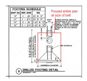
Figure 2-1: Drilled Footing as Designed
