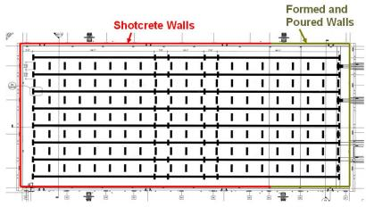
Figure 2-4: Plan View of Wall Placement Methods
