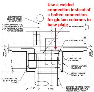
Figure 2-5: Glulam Column Connection Detail
