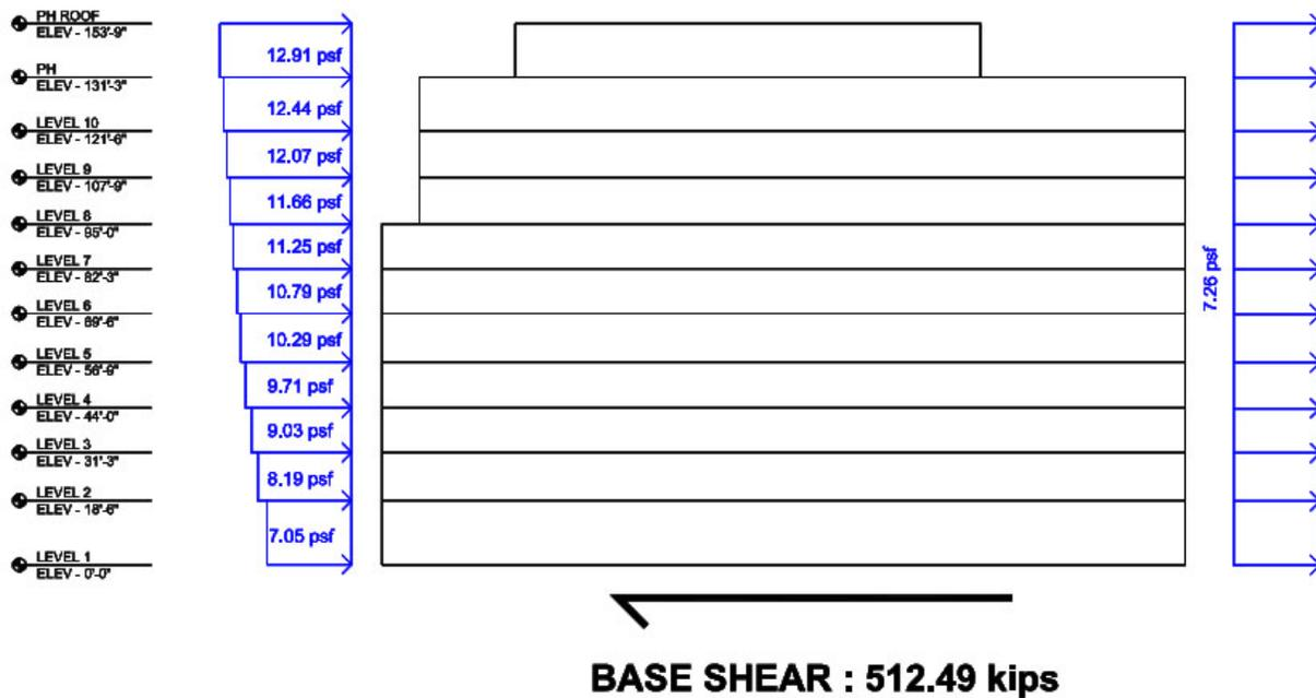
Figure 11: N/S Wind Load Diagram
