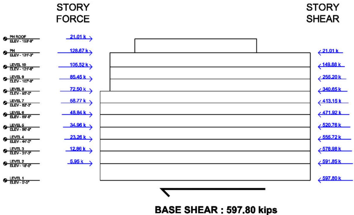
Figure 13: Seismic Force Diagram
