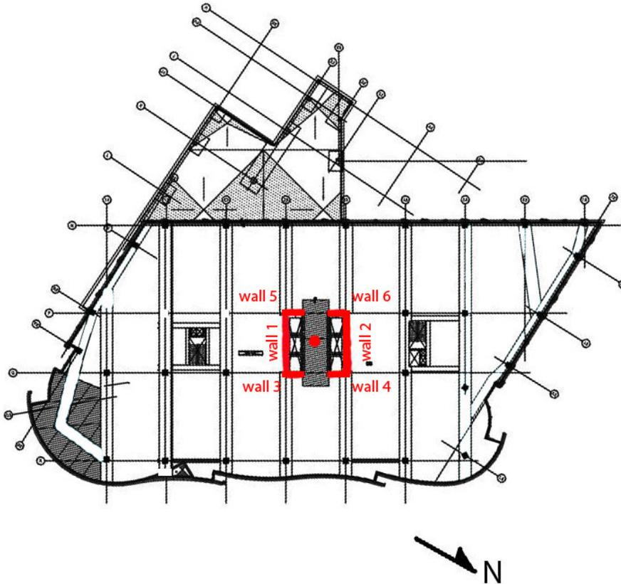
Figure 16: Lateral System (shear walls) with Labels
