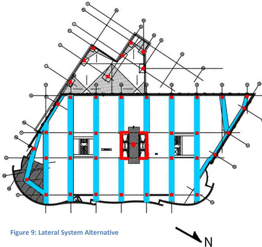
Figure 9: Lateral System Alternative
