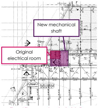
Figure 6 The proposed mechanical shaft
