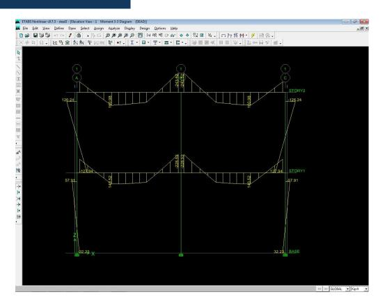
Figure 18.2 ETABS model of the Composite System showing the maximum moment on the beam.
