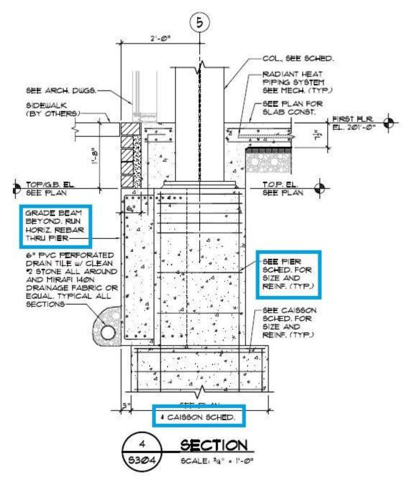
Figure 6 A section cut of a drilled caisson foundation. Courtesy of Highland Associates
