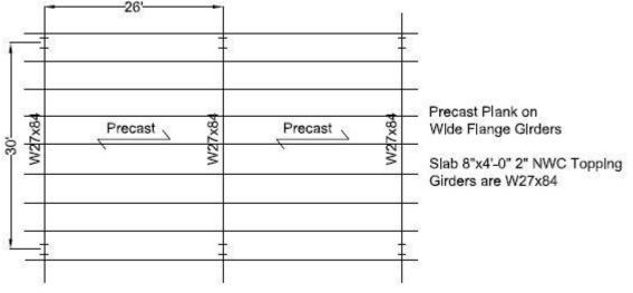
Figure 21 Precast Plank on wide flange girders
