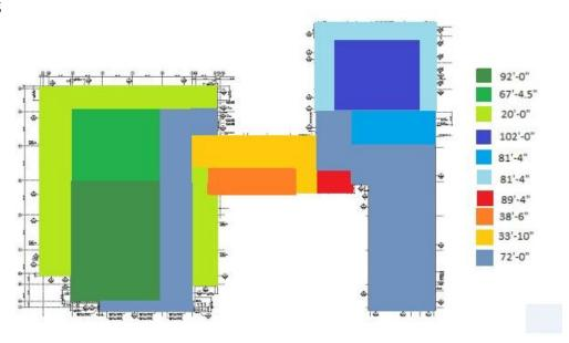
Figure 8 Plan showing the different roof heights; the darker, the higher.
