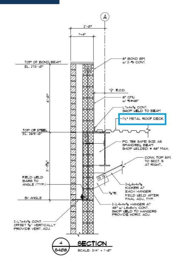
Figure 9 Typical roof section cut showing the roof deck. Courtesy of Highland Associates
