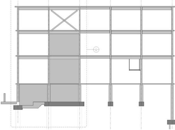
Figure 17: Shear wall at column line 15
