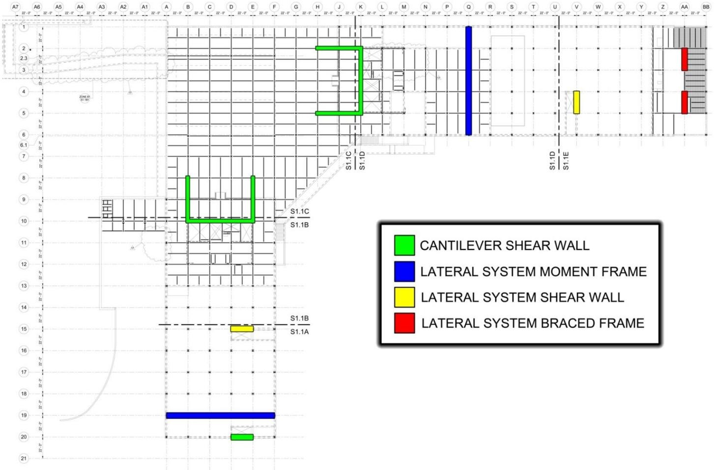
Figure 15: First floor lateral system elements
