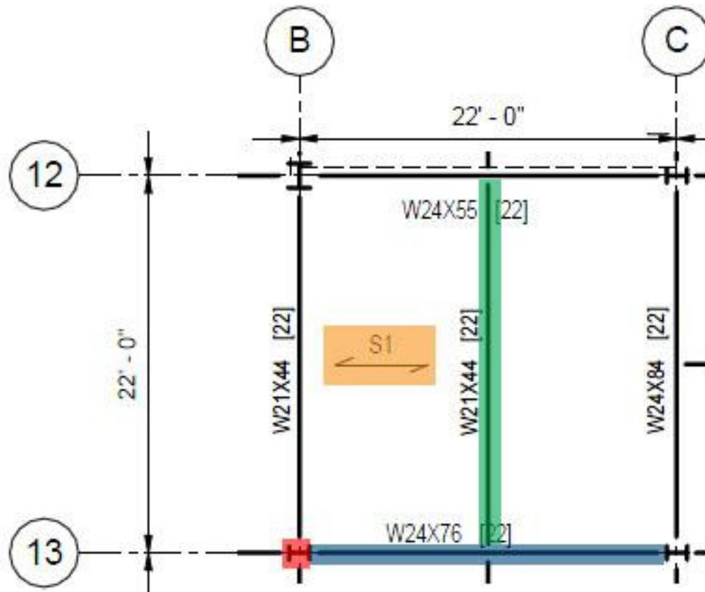
**Figure 13:** Figure of typical interior gravity frame used for spot checks. Orange: composite metal deck, green: composite beam, blue: composite girder, and red: column.
