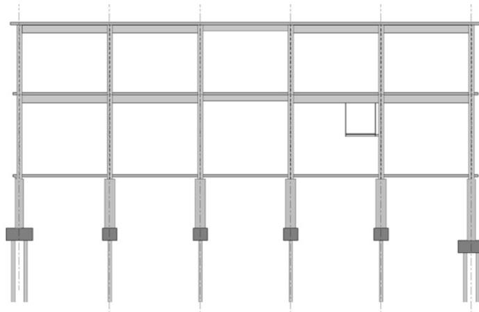
Figure 18: Moment frame at column line 19
