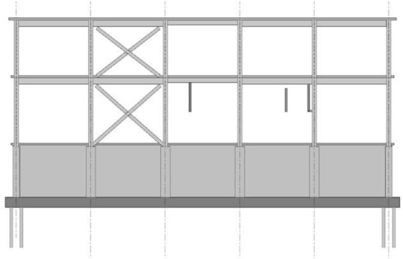
Figure 19: Braced frame at column line 20
