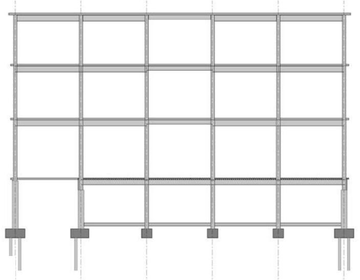
Figure 21: Moment frame at column line Q
