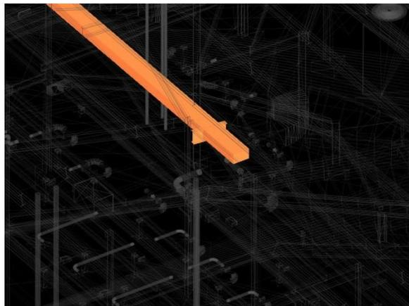
Figure 109. Exhaust Duct and Stub Cantilever Clash
