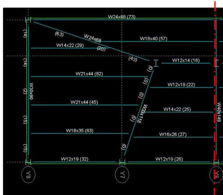
Figure 69. Structural Design of the Loft Level from RAM
