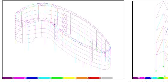
Figure 33a: Perimeter truss virtual work
