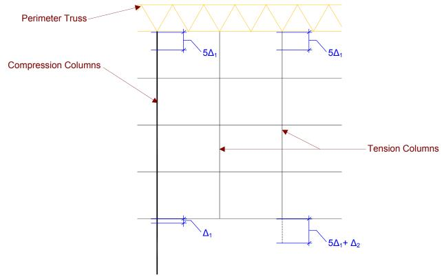
Figure 38: Column deformation incompatibility
