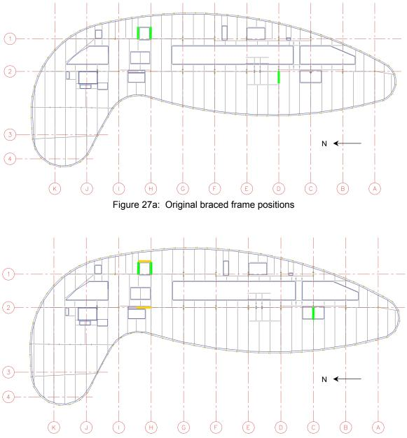
Figure 27b: New braced frame positions
