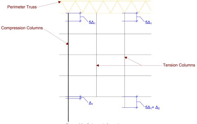
Figure 23: Column deformation
