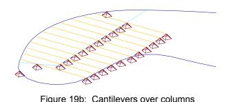
Figure 19b: Cantilevers over columns
