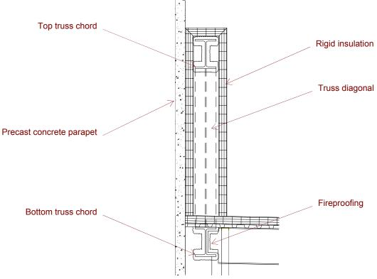
Figure 24: Perimeter truss insulation
