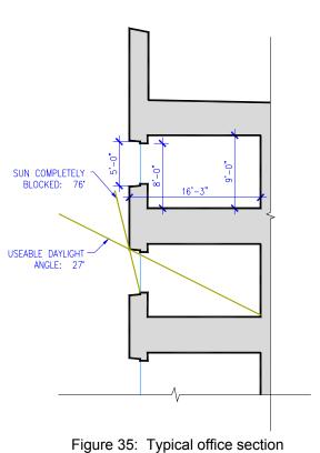
distance of 1'-4" from the façade face. This "deep façade" approach creates a buffer zone which filters glare and blocks high sun angles. Figure 35 is a section through the typical office showing room dimensions and two key solar angles.
