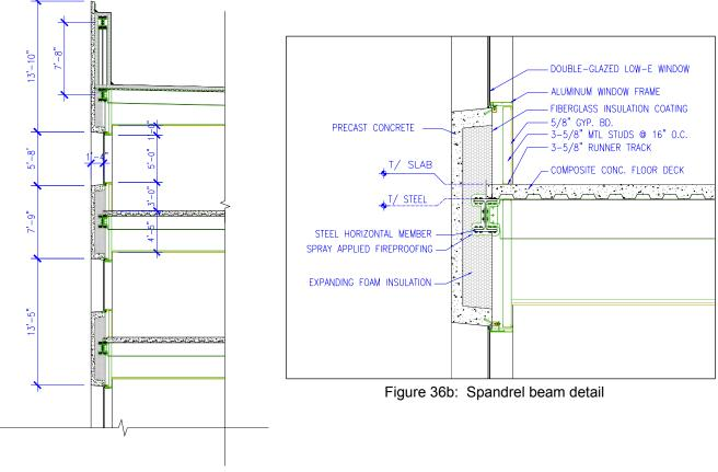
Figure 36a: Curtain wall section
