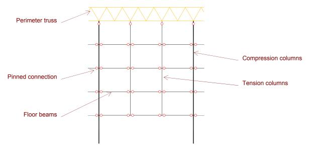
Figure 22: Pinned connection schematic
