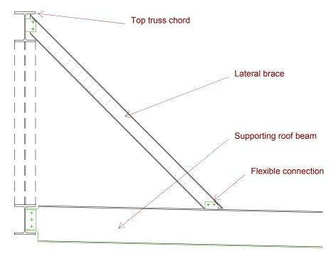
Figure 26: Truss lateral bracing
