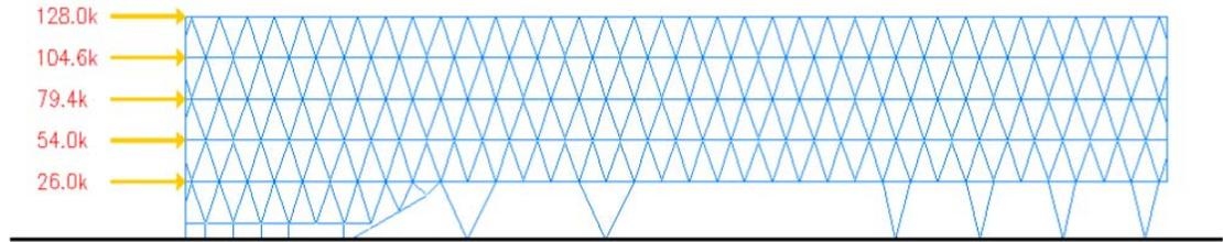
Seismic shear in both directions.
