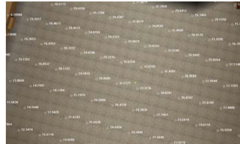
Between 20 and 35 footcandles on the float with the pendants on 100%.
