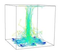
fine mist that exhibits gas-like dispersion behaviors to absorb the energy of the fire and act as a flooding agent to extinguish fires. Their use of computer simulation models has made it easier, faster, and more affordable for water-mist technology to be developed. Through the use of a computational fluid
