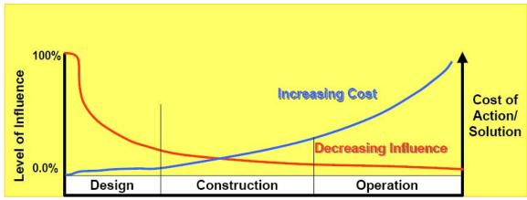
\*Shows a direct relationship between level of influence associated during the design aspect of a project in reference to an increasing cost to fix, replace, and rectify a problem as a projects duration increases over time.
