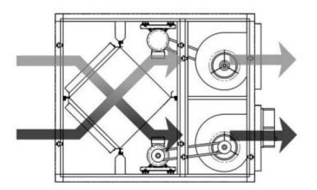
Figure 5: Membrane Heat Exchanger Schematic
