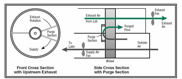
Figure 4: Desiccant Wheel Schematic
