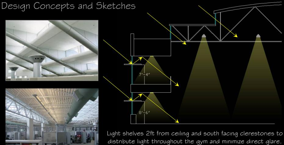
distribute light throughout the gym and minimize direct glare. Fixtures are dimmable-high bay compact fluorescent controlled by photosensors.
