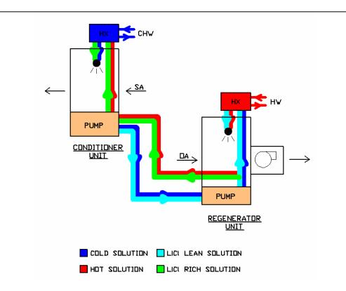
**Figure 3** Kathabar System Schematic
