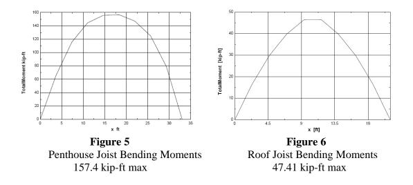
of 2525 plf. Referring to Table 8, the maximum plf that occurs at any time along the joist is 1,824. This joist is found in the <u>PCI Design Handbook 6<sup>th</sup> Edition page 2-42</u>. Because the joists are fixed to the slab they are supporting, it is assumed that they are braced along their entire length.
