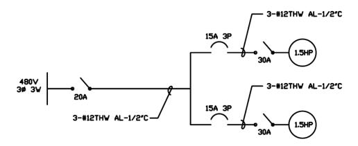
**Figure 10** Regenerator Unit Branch Circuit
