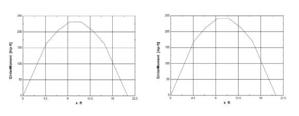
Figure 8 Penthouse Girder R1 Bending Moments 231 kip-ft max
