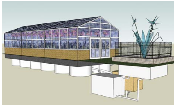
Figure 36: Constructed Wetlands Greywater System Created in Google SketchUp
