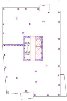
the most common reinforcing is #5 bars at 12" o/c at the top and bottom of the slab going both directions. The bottom of the slab is left exposed over the living rooms and bedrooms of the condominium units. The typical floor plan can be seen on the left.
