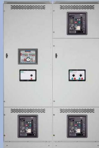
Two modules—a Single Generator with Master Control and a Dual Generator with redundant control—comprise switchgear for a three engine power system. Three engine systems requiring redundant master control would need three modules—Master Control, Single Generator and Dual Generator.
