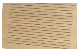
Wall Material Wood Acoustical Panels Reflectance = 0.44
