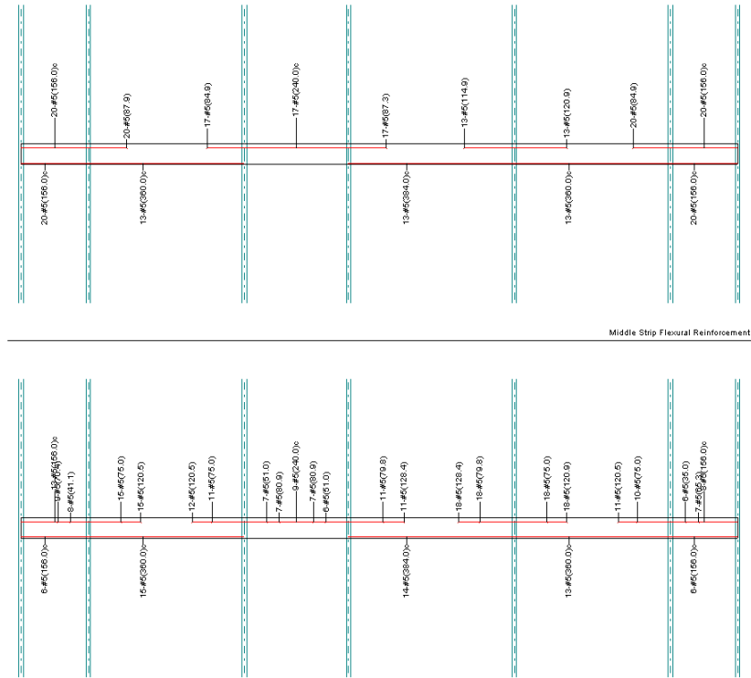
Figure 30 –Reinforcement for Typical Cooling Tower Width
