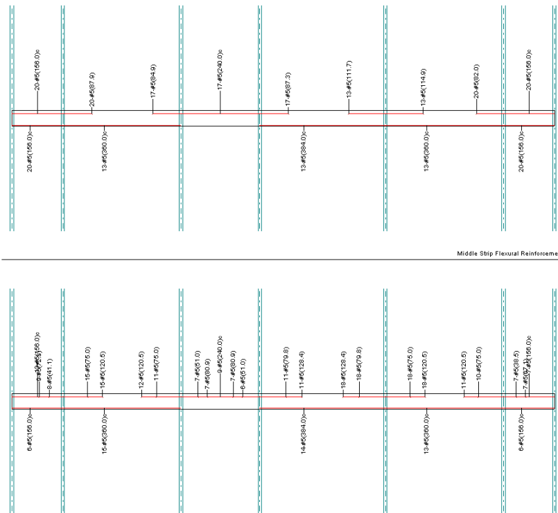
Figure 27 –Reinforcement for Typical AHU Width
