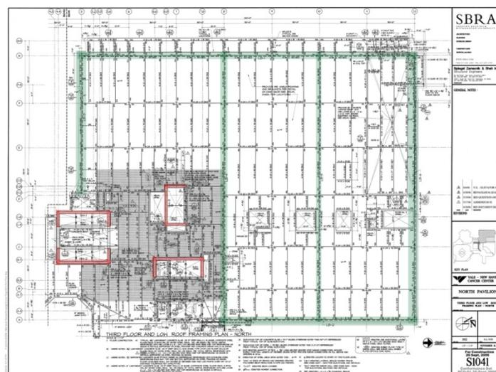
Figure 1a: Typical Framing Plan for Levels 1-5. Green denotes Moment Frames; Red denotes Shear Walls.
