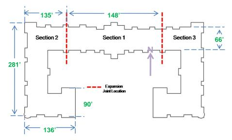
The relocation of expansion joints is needed due to the irregular configuration of the building. Two main problems related to seismic performance that may result are:
