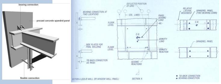
There is a problem however, with the connections of corner panels and connections. They must be designed to permit panels to slide past one anther with minimum damage.
