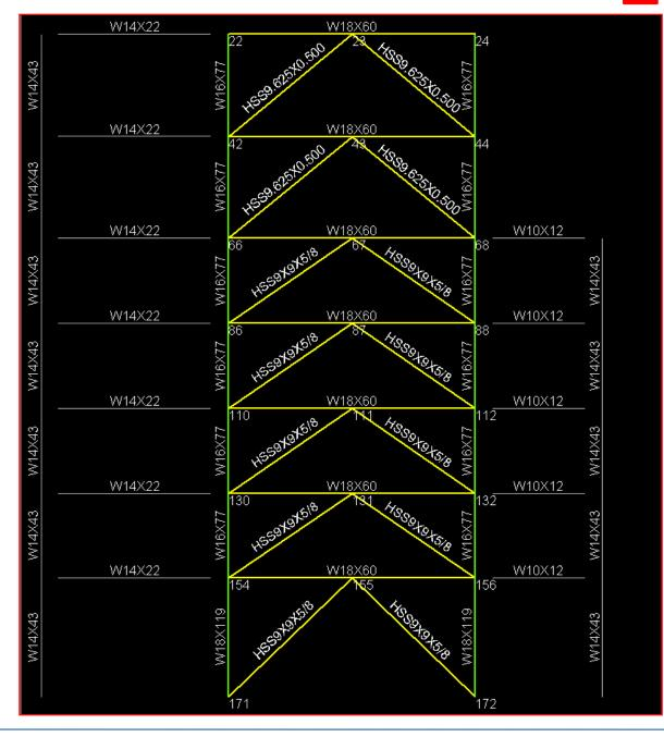
RAM Diagram: Section 1 7th Floor Plan
