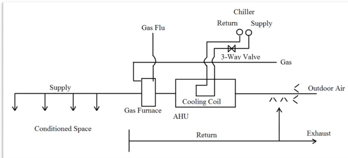
• Figure 20 – Schematic of Chiller Based Mechanical System
