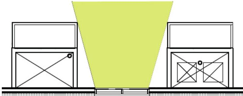
• Figure 18 – Mechanical Ducts Limit Light into Fitness Center
