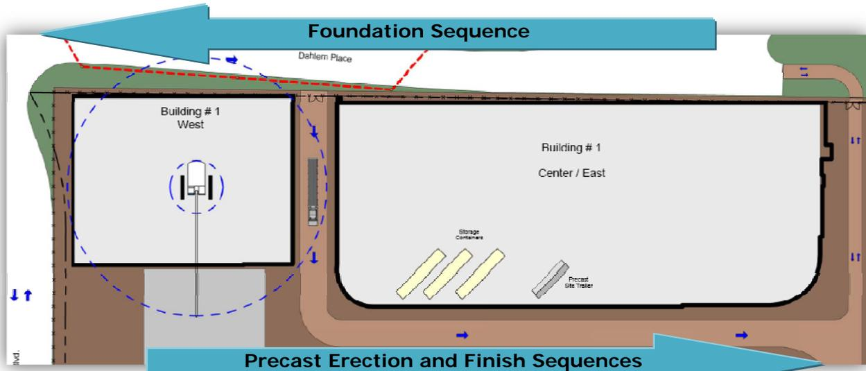
• Figure 6 – Site Plan with Sequencing Illustrations
