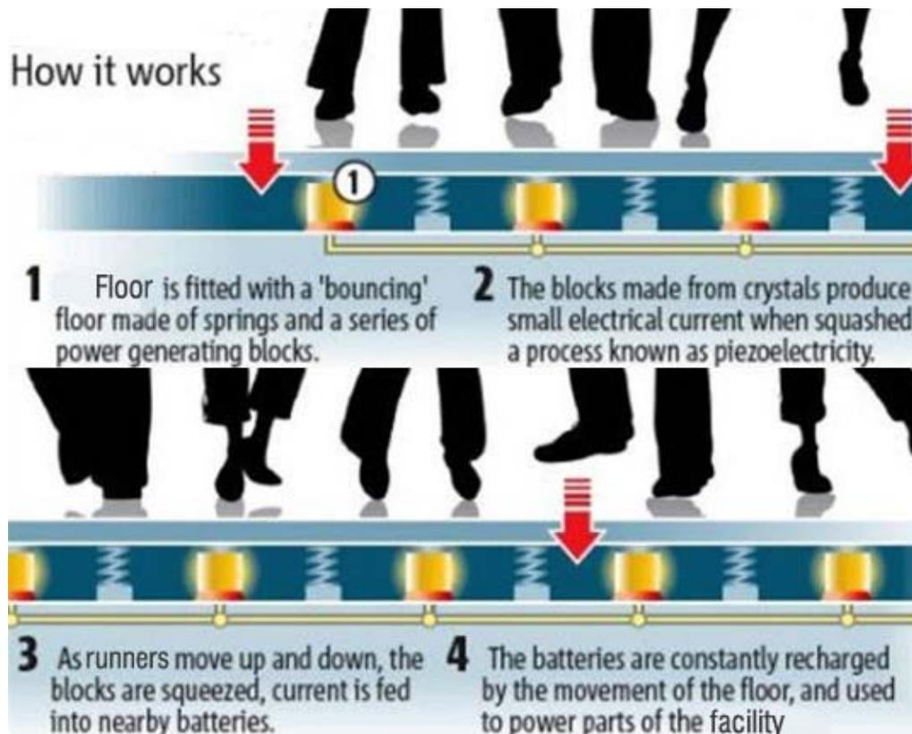
• Figure 12 – Piezoelectric Floor Tile Description
