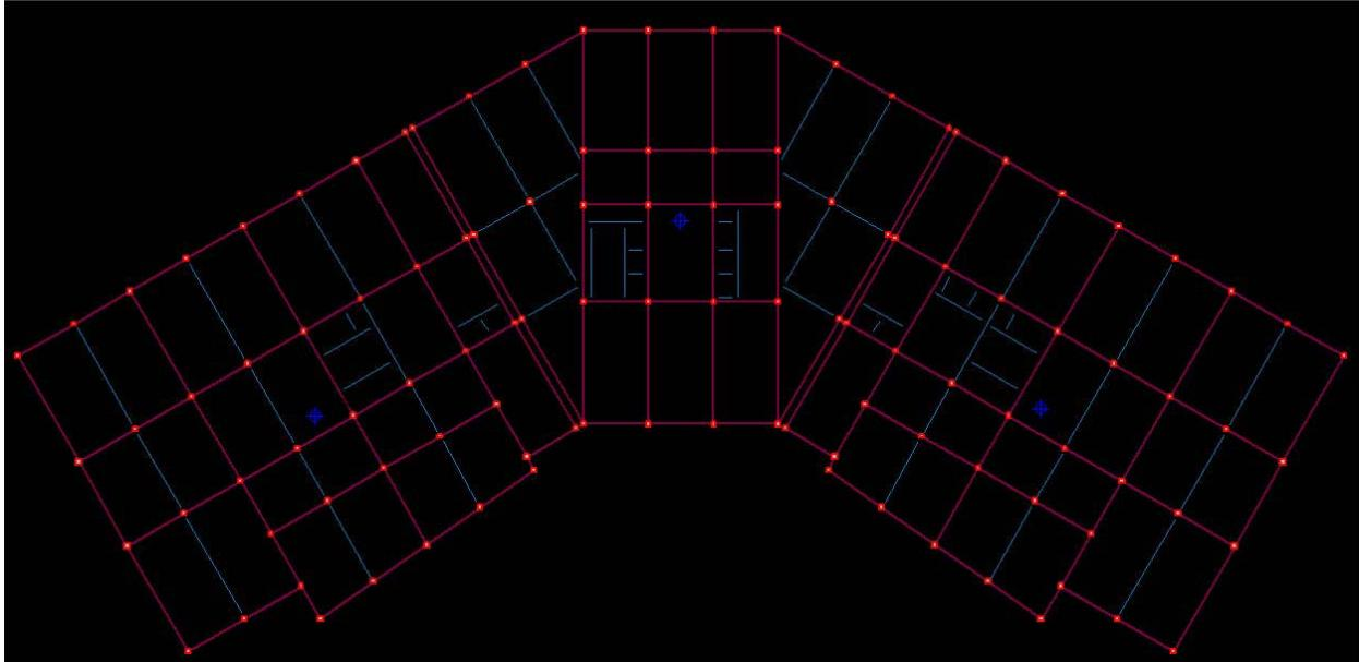
Figure 17: Centers of Rigidity of new concrete design
