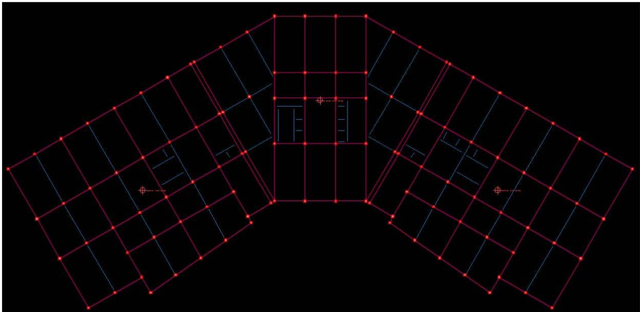
Figure 16: Center of Mass of concrete new design
