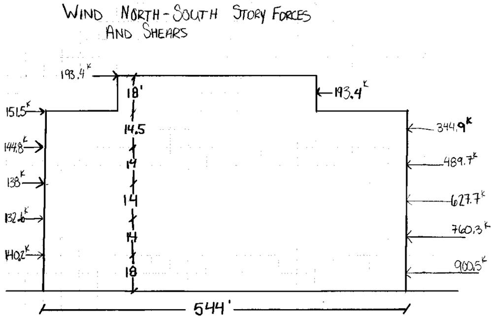
Figure 7: Wind North-South Story Force and Shear Diagram
