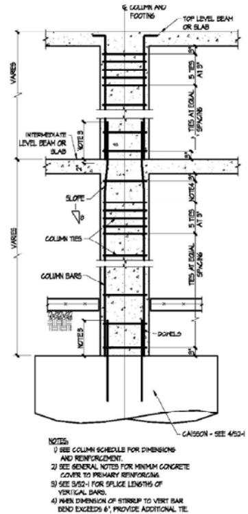
① COLUMN BAR BENDING DETAIL
