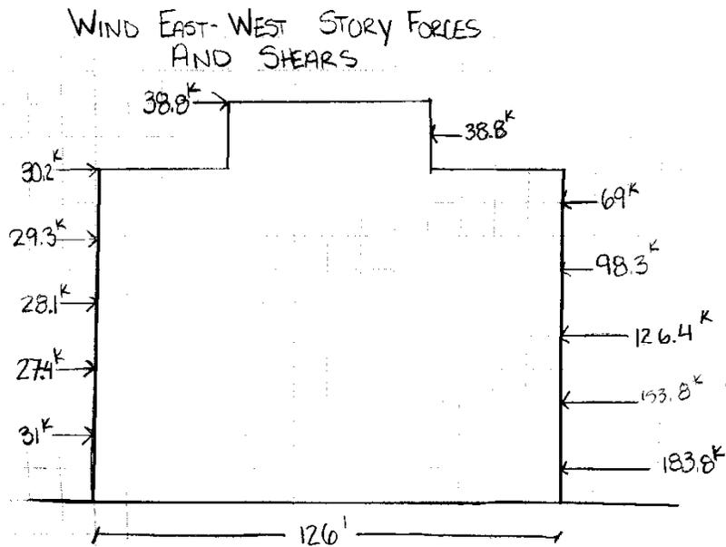
Figure 8: Wind East-West Story Force and Shear Diagram
