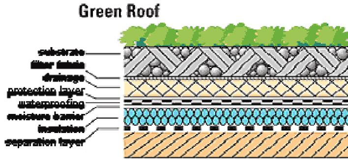
Figure 27: Green Roof Detail courtesy of [www.deq.state.mi.us/documents/deq-ess-p2-p2week-greenroofreources.doc](http://www.deq.state.mi.us/documents/deq-ess-p2-p2week-greenroofreources.doc)
