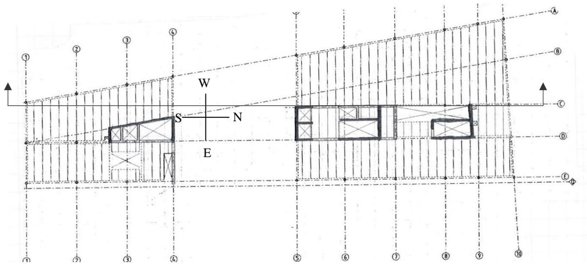
Figure 4: Typical framing plan for floors 1 - 4
