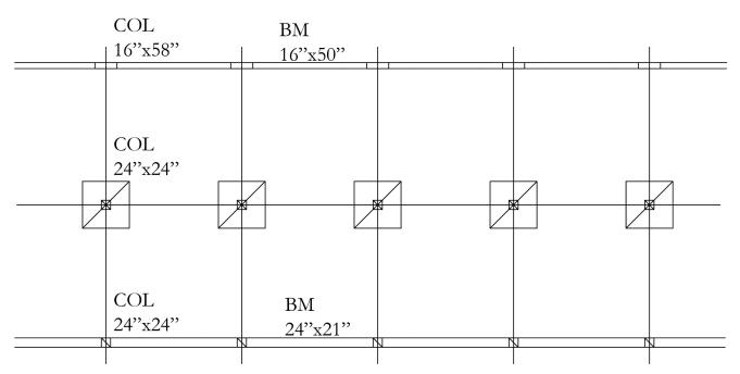
Figure 4: Typical Bays with Column and Beam Indentification
