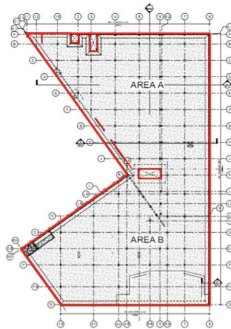
Figure 9: Typical Shear Wall Locations in Tower Levels
