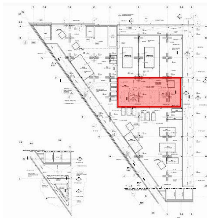
Figure 26: Area Under Cooling Towers Considered for Acoustic Analysis
