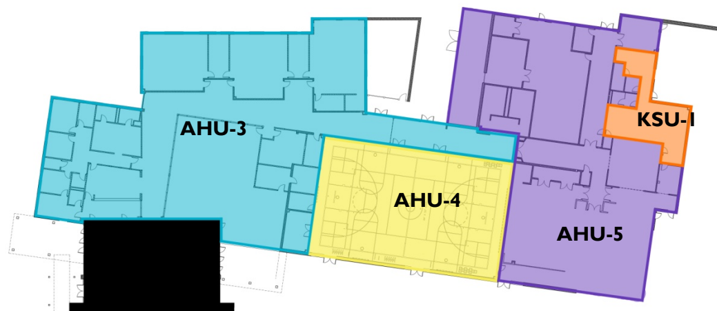
Figure 2: Wing B AHU Air Distribution Schematic
