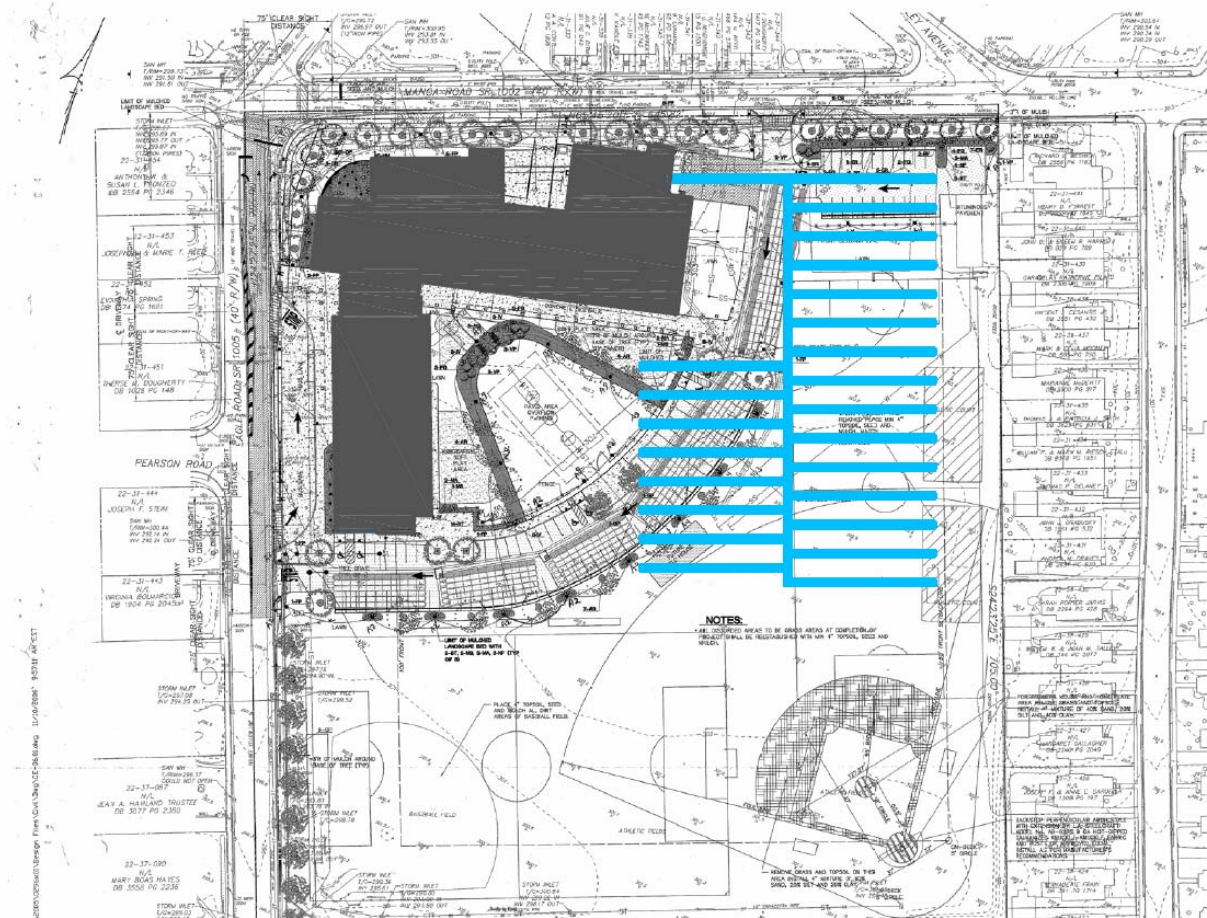
Figure 20: Vertical Borefield Layout
