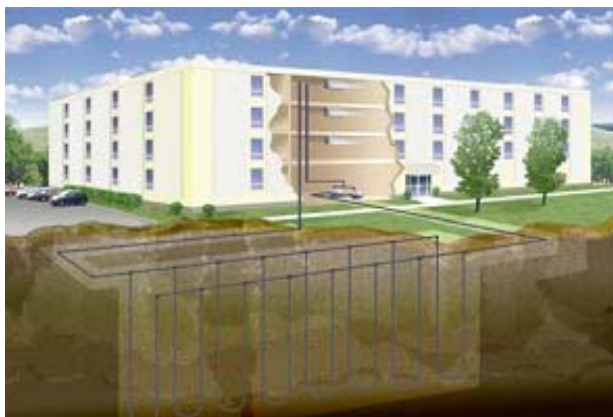
Figure 10 –Conceptual Vertical Loop System
