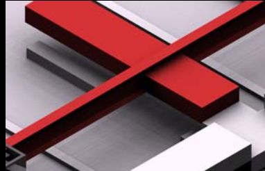
30 x 132 beam clashing with a 24" x 80" duct (recreated in Navisworks)
