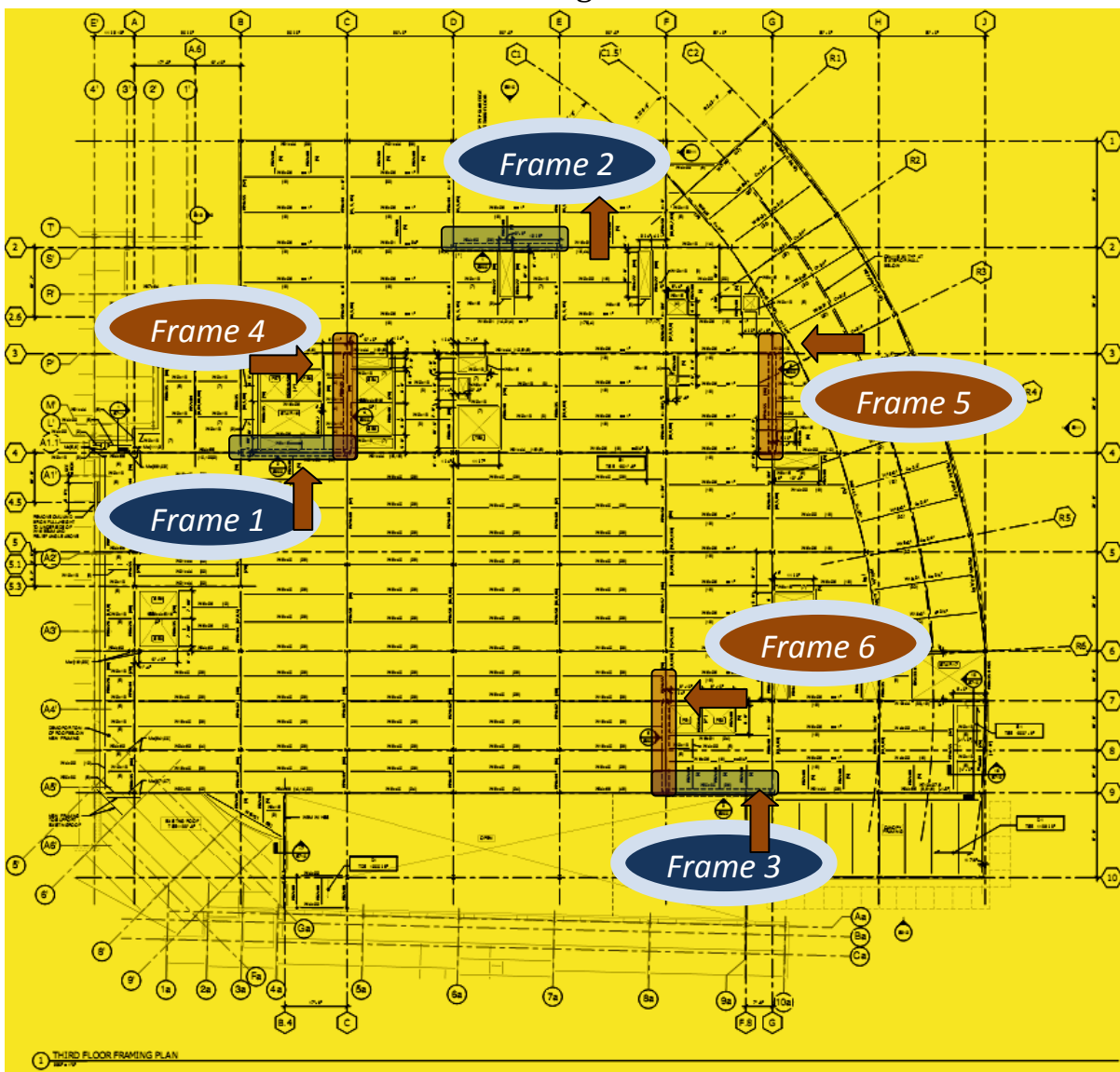
Figure 3.1: Third floor framing plan with braced frame locations shown
