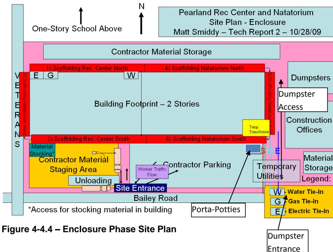
**Figure 4-4.4 – Enclosure Phase Site Plan**
