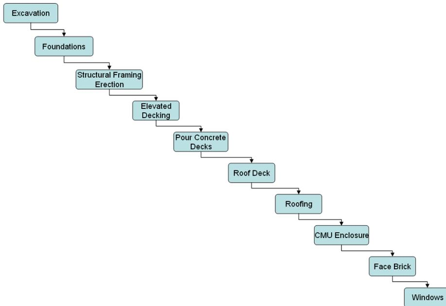
**Figure 5-2.2 – Structural and Enclosure Trade Construction Sequence**
