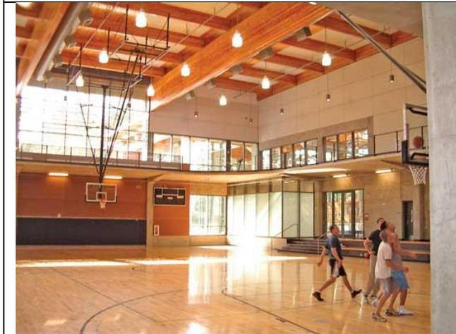
**Figure 6-1.2 - Gymnasium with glulam structural system.** Courtesy of Structure Mag
