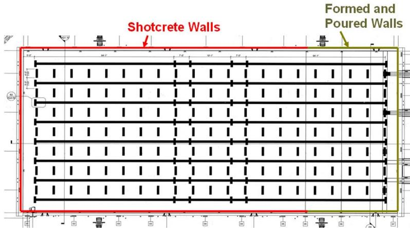
Figure 2-4: Plan View of Wall Placement Methods
