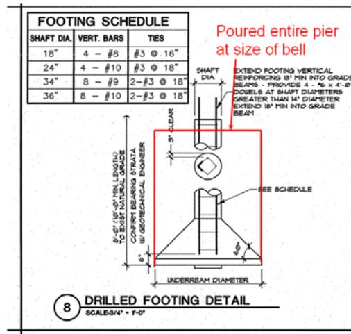
Figure 2-2: Modified Drilled Footing
