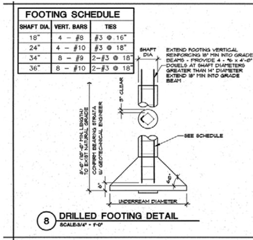
Figure 2-1: Drilled Footing as Designed
