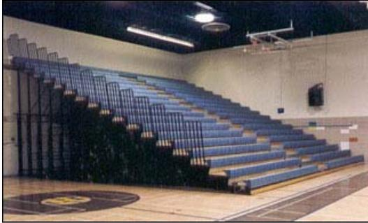
Figure 4-1: Telescoping bleachers. Courtesy of Hahn Enterprises
