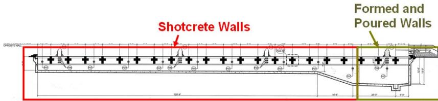
Figure 2-3: Section View of Wall Placement Methods
