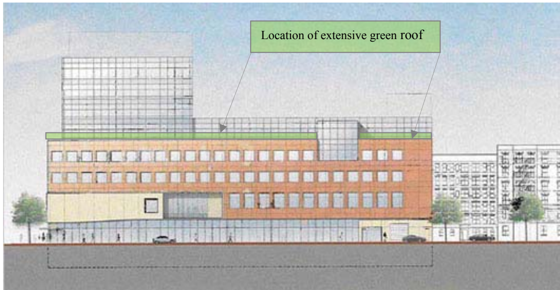
Figure 59: Location of Redesigned Extensive Green Roof
