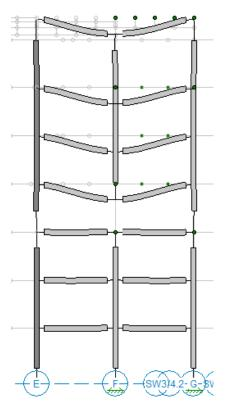
Figure 7.17 – Deflected shape of a portion of the frame that ran along column line when column F5 was removed at the 4<sup>th</sup> story.
