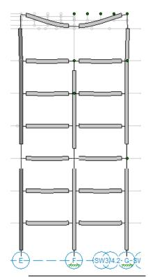
Figure 7.19 — Deflected shape of a portion of the frame that ran along column line when column F5 was removed at the 7<sup>th</sup> story.
