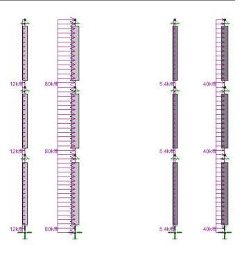
Figure 8.2 —Elevation view all four columns investigate in the ELR analysis
