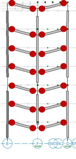
Figure 7.26 – Plan Location of Column A.2-2.4 Plastic hinge
