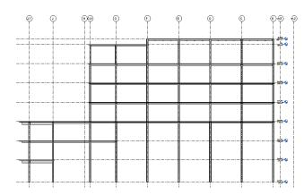
4.6 shows the irregular and often interrupted configuration of column line B. For these reasons, a moment frame was added along column line C, which is more regular. Due to the larger forces resisted by the North-South direction frames, which were due to the larger wind surface area, another frame line was added at column line E. Column line G.9 was also selected as a frame line because it runs continuously from base to roof, whereas column line J terminates at below the fourth level.
