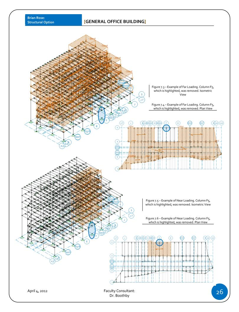
Figure 7.7 illustrates the different loadings in the progressive collapse model. These loads were broken into near and far load cases. The load combinations, shown in Figure 7.4, combined these load cases with the appropriate factor. The magnitude of the near and far loads were the same, they were only separated so that the different load factors could be applied. For instance, 100 psf distributed loads were used in both the "Far Typ Live" and Near Typ Live" load cases.
