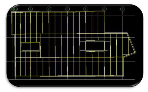
Figure 4.6 – Deflected shape of the  $5^{th}$  Floor when the direct wind load was applied to the South Facade
