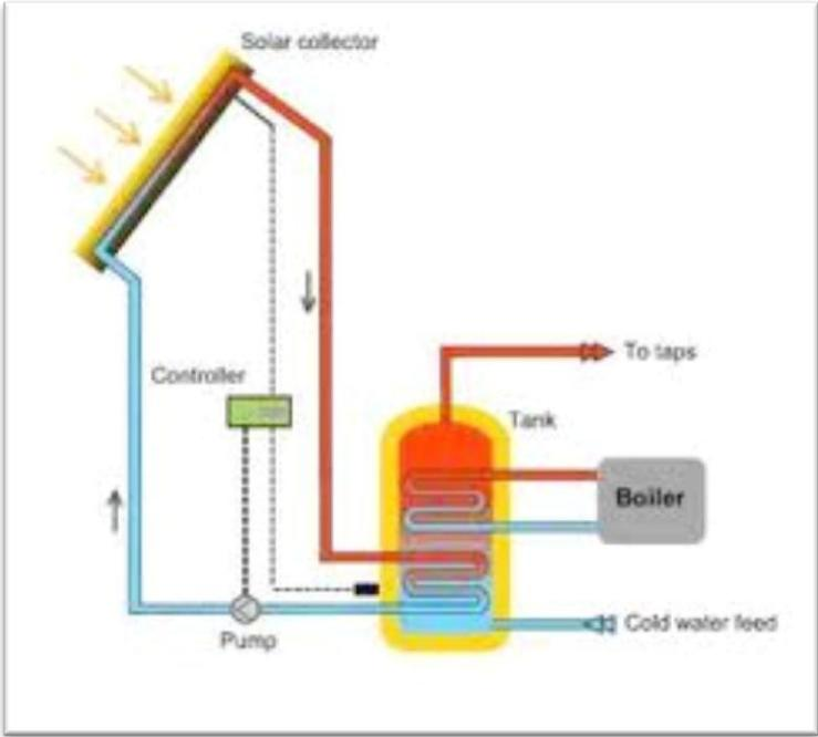
Figure 3 - Solar Thermal Storage System
