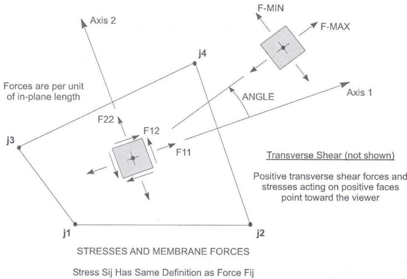
**Figure 27** Diagram from the CSI Analysis Reference Manual displaying how ETABS reports shell forces.
