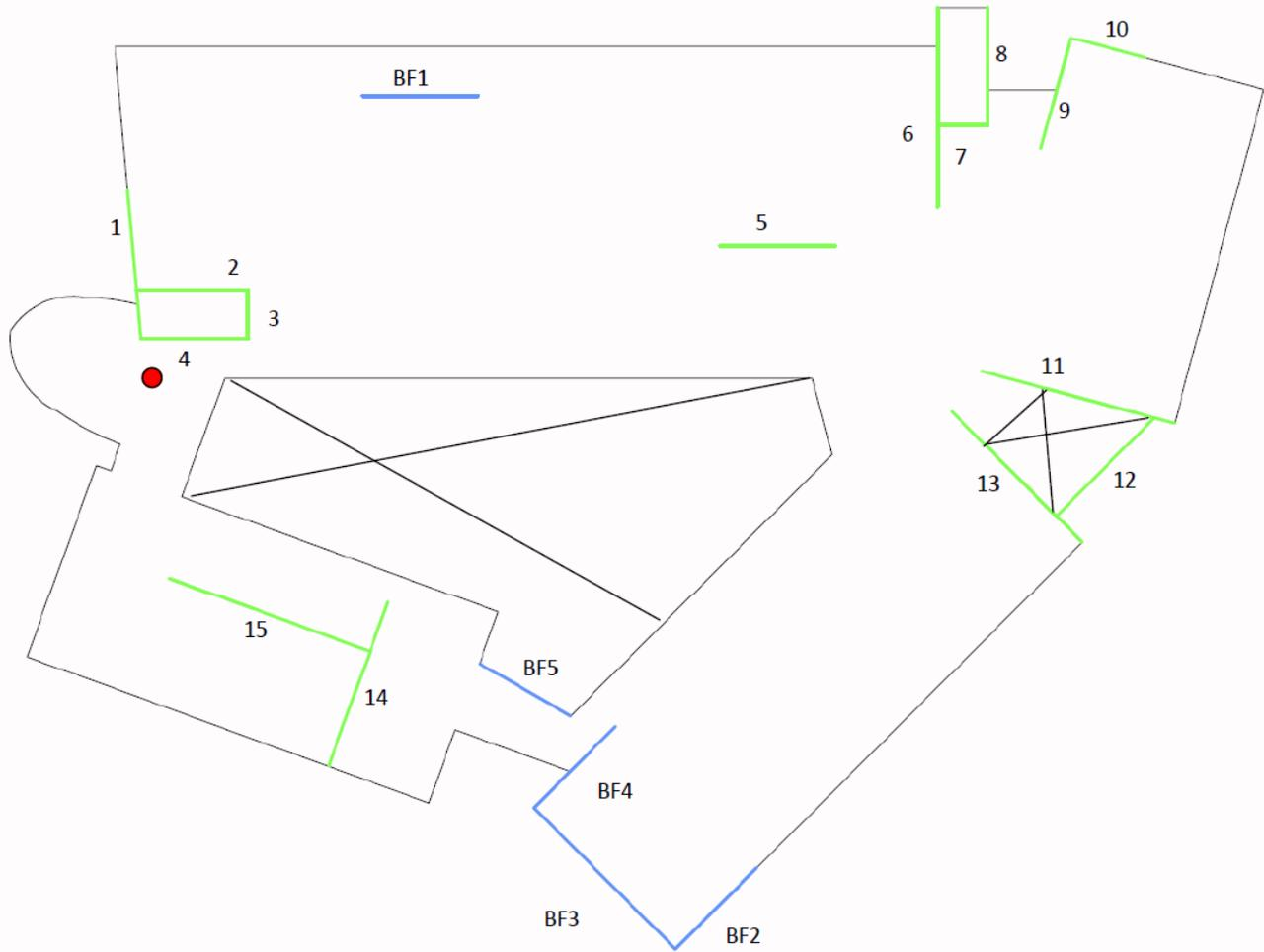
**Figure 8** Floor plan with shear walls indicated in green and braced frames (present only above Level 5) indicated in blue. All are labeled for ease of reference. Red dot is the reference location for (0,0) ft.
