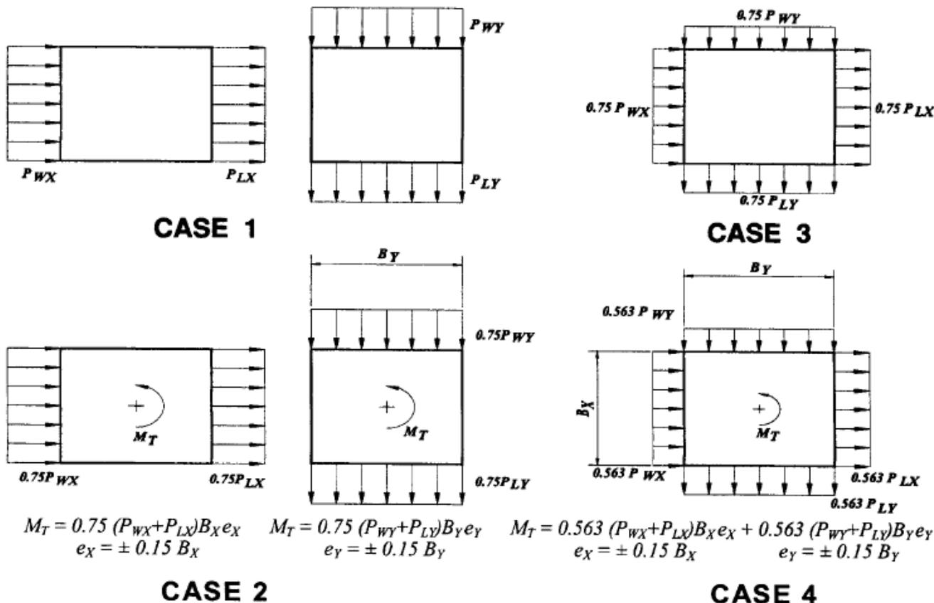
Figure 11 Torsional wind load cases from Figure 6-9 in ASCE 7-05.
