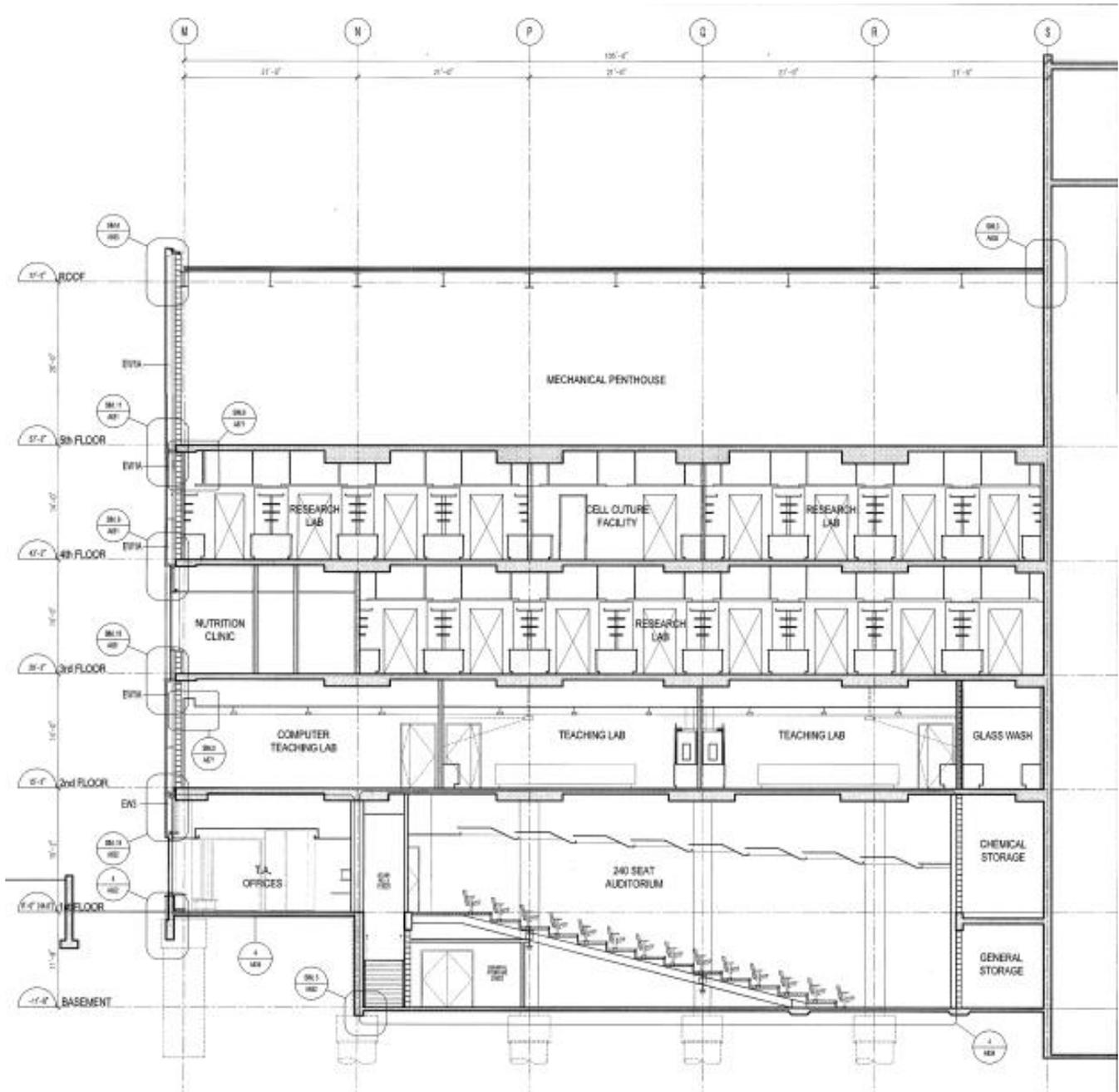
Figure D.4 Section 3 through portion of building at -45° rotation (see Figure 1), taken from 4/A402.
