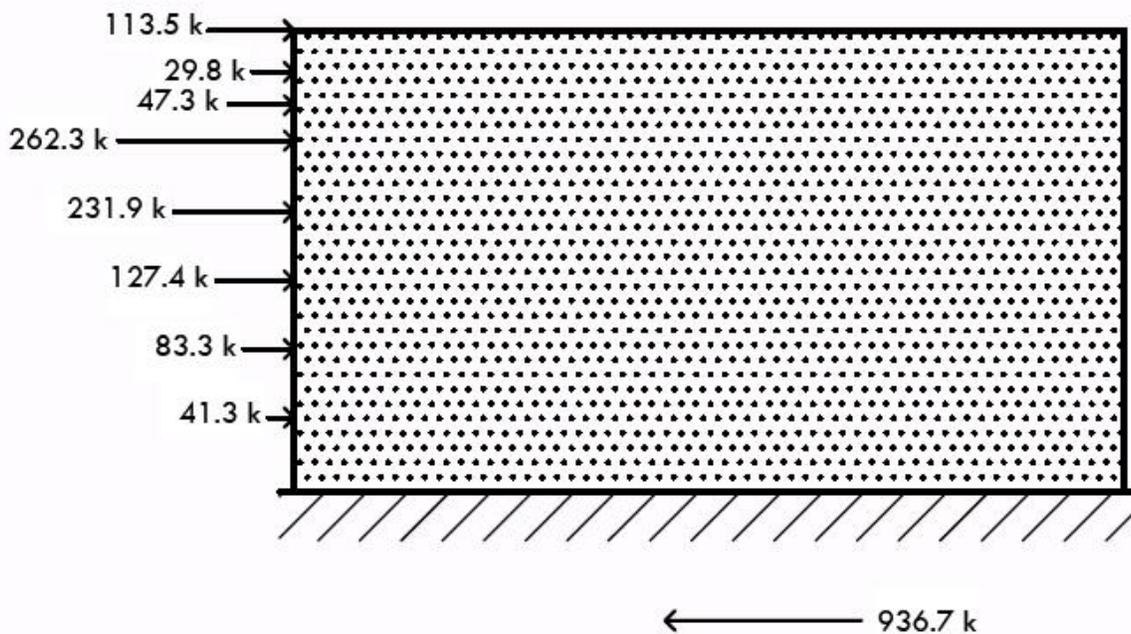
**Figure 20** List and diagram of E-W direction seismic forces as calculated by the Modal Response Spectral Analysis Procedure for the Rigid Diaphragm periods.
