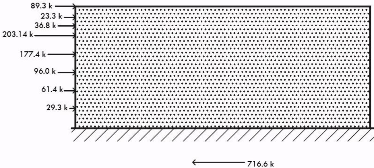
**Figure 19** List and diagram of N-S direction seismic forces as calculated by the Modal Response Spectral Analysis Procedure for the Rigid Diaphragm periods.
