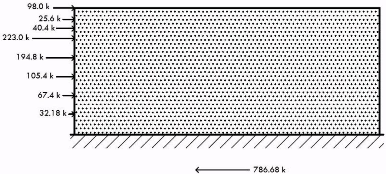
Figure 17 List and diagram of N-S direction seismic forces as calculated by the Equivalent Lateral Force Procedure.
