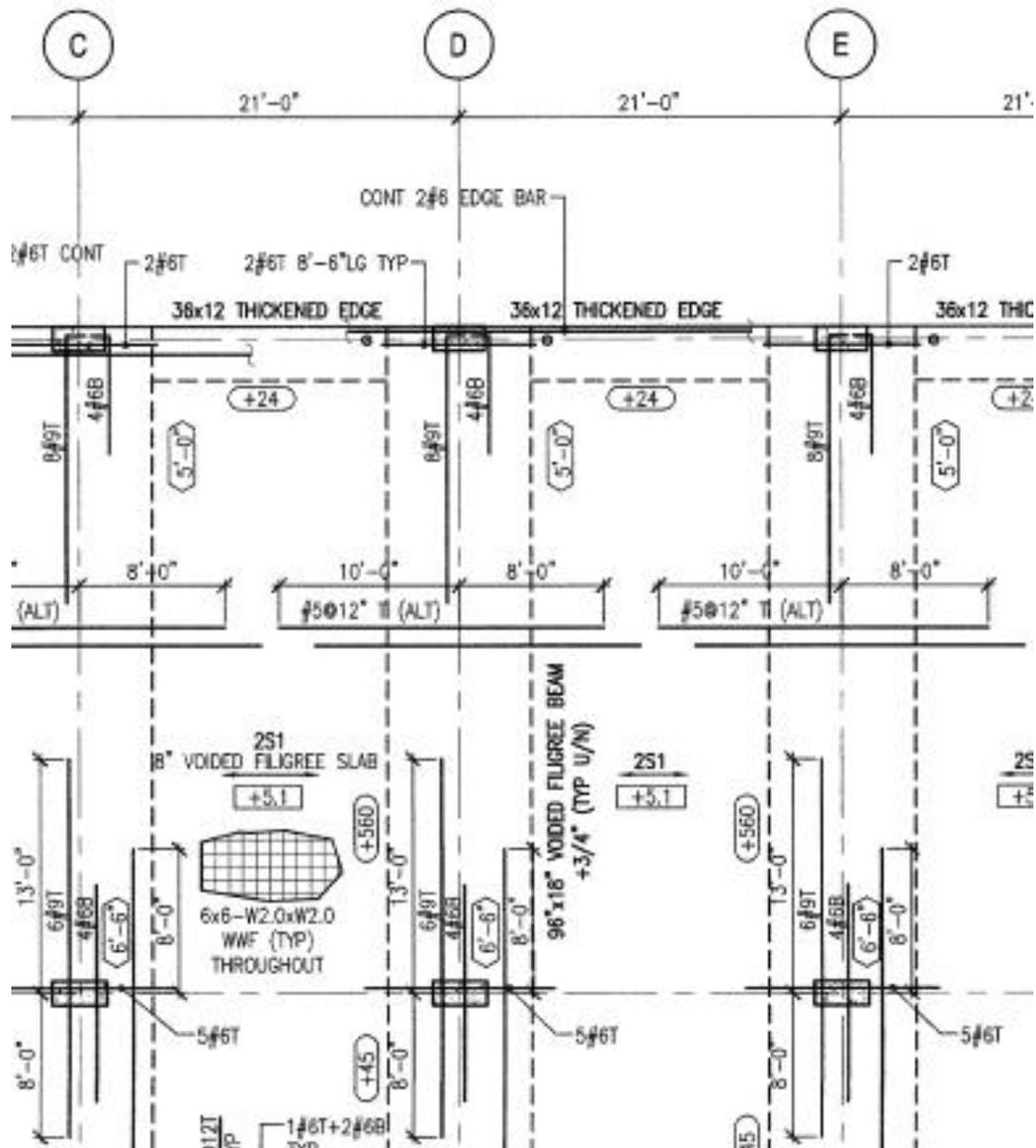
**Figure D.6** Enlarged floor plan for a typical bay in the laboratory wing, taken from S202 (levels 2 through 4 are identical, and reinforcing is only displayed on level 2). Slab design moments are boxed (k-ft/ft), beam design moments are enclosed in an oval (k-ft), and the location of the first void in the beams with relation to the face of columns is enclosed in a prism-like shape.
