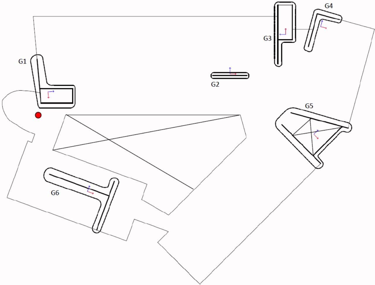
**Figure 24** Floor plan showing shear wall pier labels and axes used to obtain moment results. The red axis corresponds to ETABS' "V2" axis, and the blue axis corresponds to ETABS' "V3" axis. Red dot is considered (0,0) ft location.
