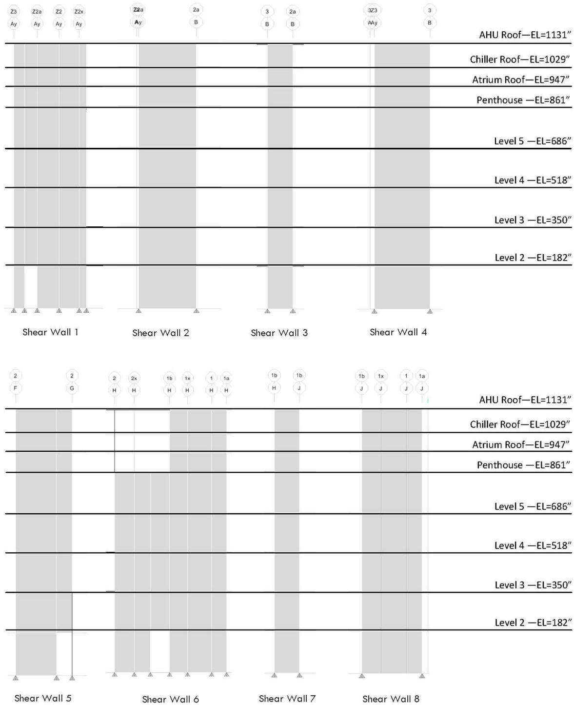
Figure 9 Shear wall elevations from ETABS model.
