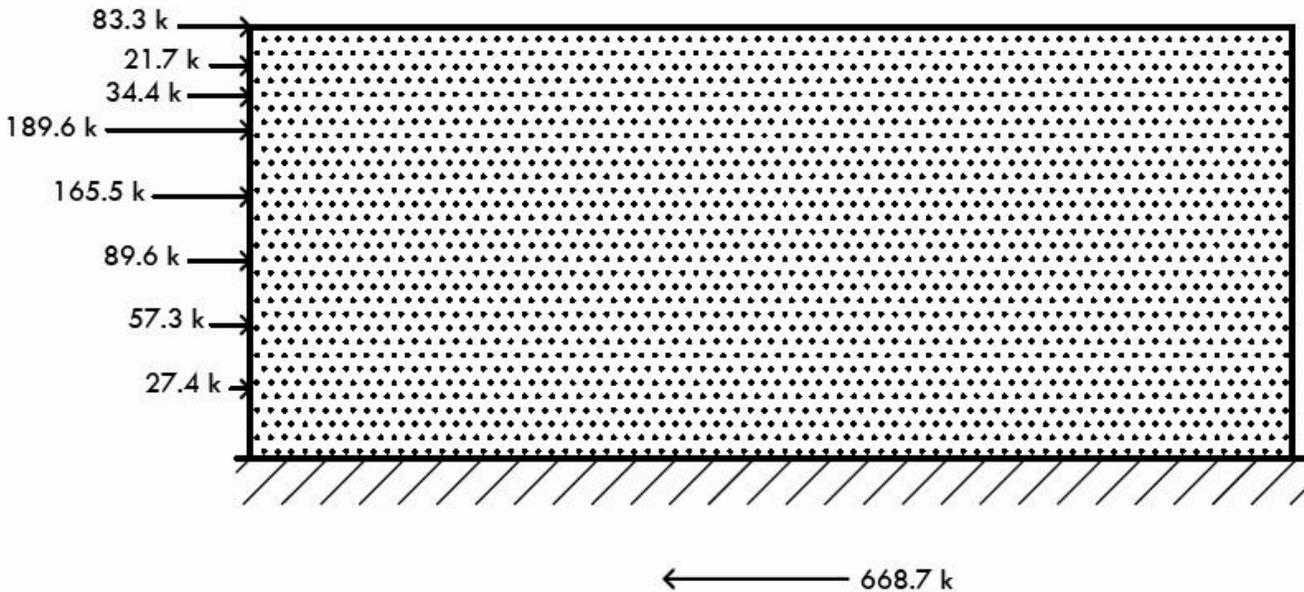
**Figure 20** List and diagram of N-S direction seismic forces as calculated by the Modal Response Spectral Analysis Procedure for the Semi-Rigid Diaphragm periods.
