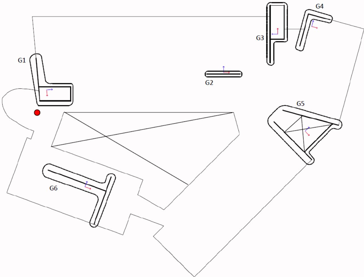
**Figure 24** Floor plan showing shear wall pier labels and axes used to obtain moment results. The red axis corresponds to ETABS' "V2" axis, and the blue axis corresponds to ETABS' "V3" axis. Red dot is considered (0,0) ft location.
