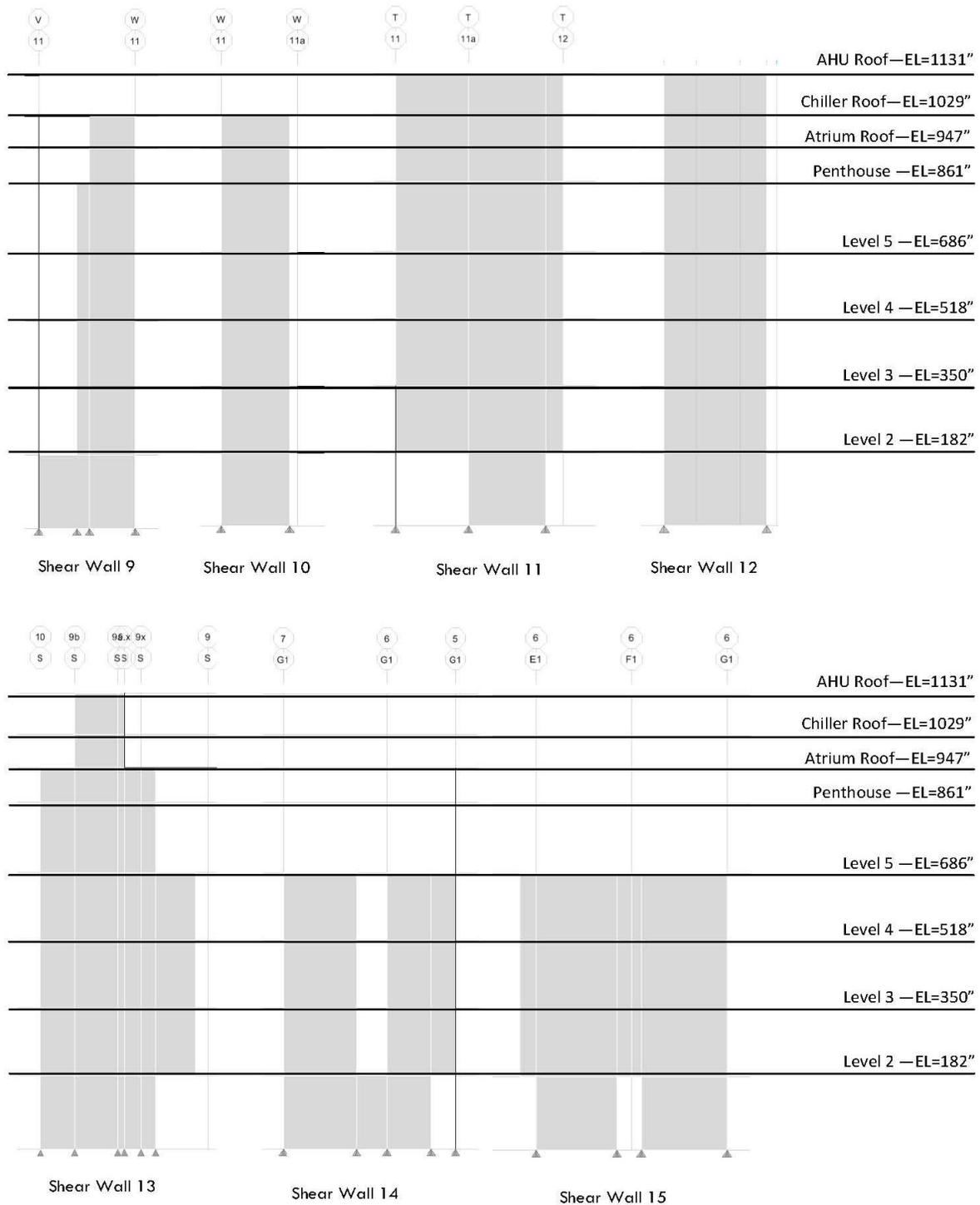
Figure 9 (cont.) Shear wall elevations from ETABS model.
