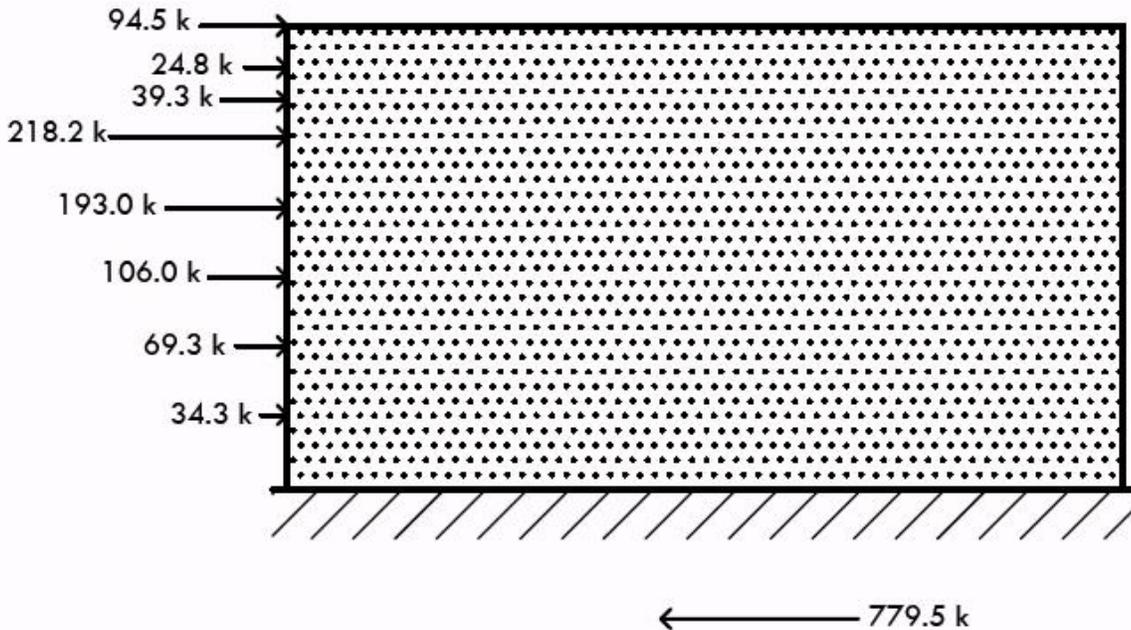
**Figure 22** List and diagram of E-W direction seismic forces as calculated by the Modal Response Spectral Analysis Procedure for the Semi-Rigid Diaphragm periods.
