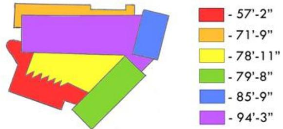
**Figure 7** Modified keyplan image from Sheets S205, & S206 showing different roof heights in relation to 0'-0"
