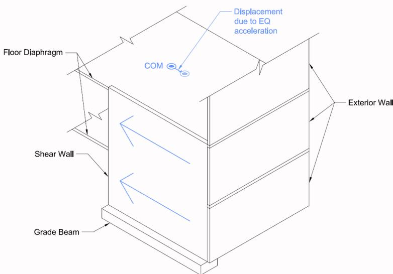
**Figure 16** Diagram of the lateral load path for a seismic load.
