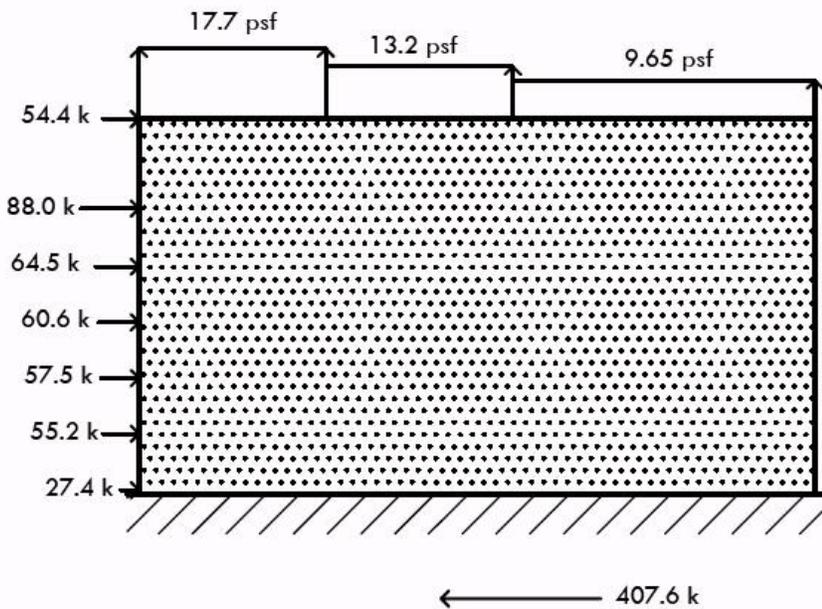
Figure 15 List and diagram of E-W direction wind forces.
