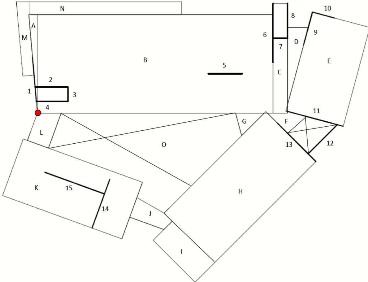
**Figure 26** Floor plan showing the areas and area labels used for the calculation of the center of mass. Areas are labeled with letters, shear walls are numbered.
