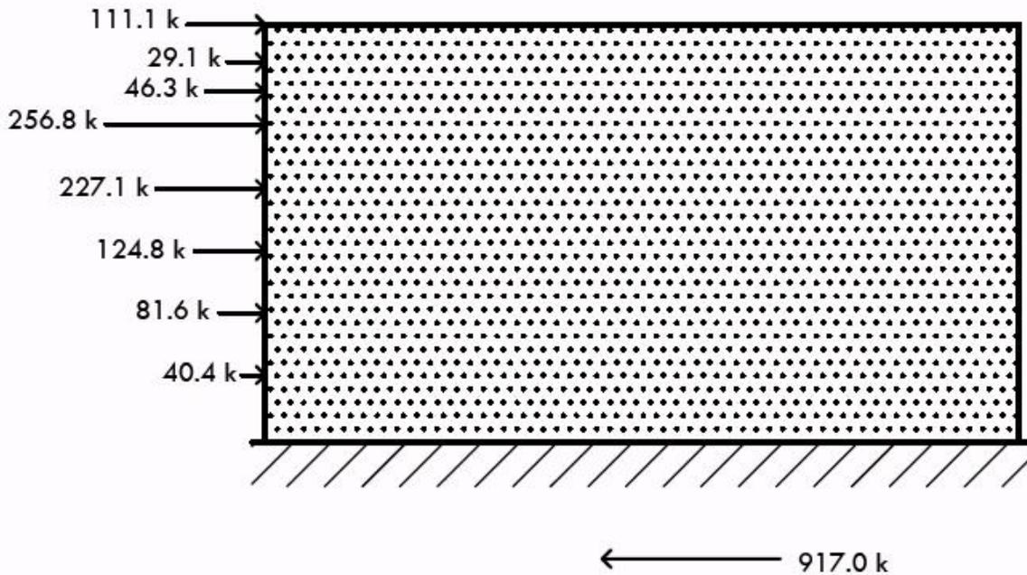
Figure 18 List and diagram of E-W direction seismic forces as calculated by the Equivalent Lateral Force Procedure.
