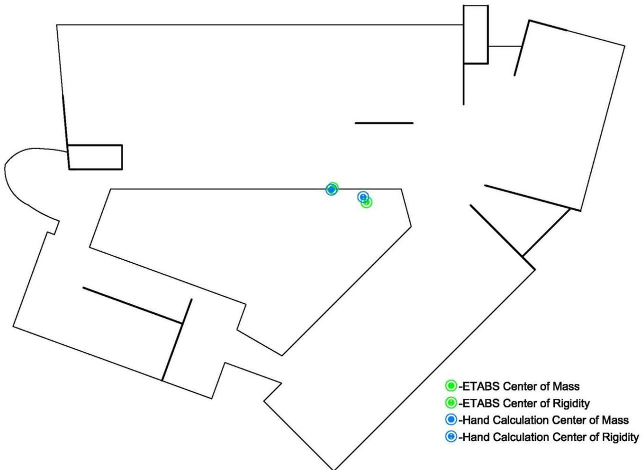
**Figure 25** 2<sup>nd</sup> Level floor plan showing the locations of COM and COR as found by ETABS and via hand calculation.
