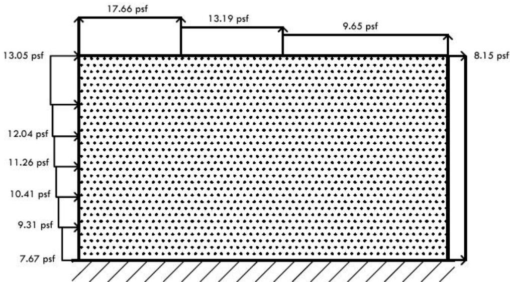
Figure 14 List and diagram of E-W direction wind pressures.
