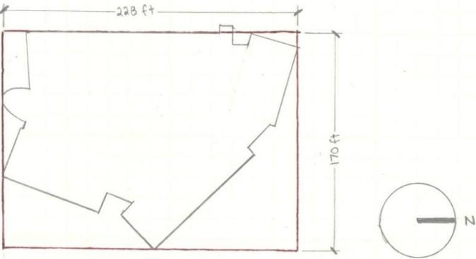
PROJECTED BUILDING DIMENSIONS FOR CALCULATING WIND FORCES
