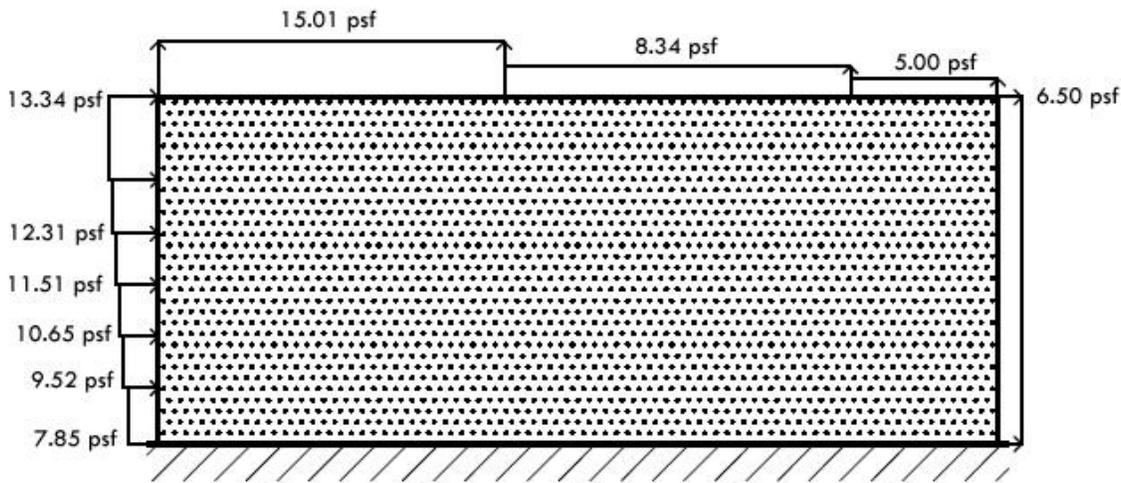
Figure 12 List and diagram of N-S direction wind pressures.
