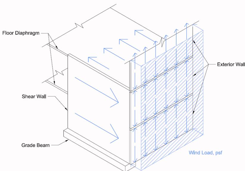
The wind loads on this building are collected by the cladding on the exterior of the building. The cladding transfers these loads to the CMU back-up walls, which are in turn anchored to the slabs with masonry dowels. This transfers the load into the slabs, which then carry the load to the shear walls. These return the loads to the foundations, and therefore to grade. This load path is illustrated in Figure 10.
