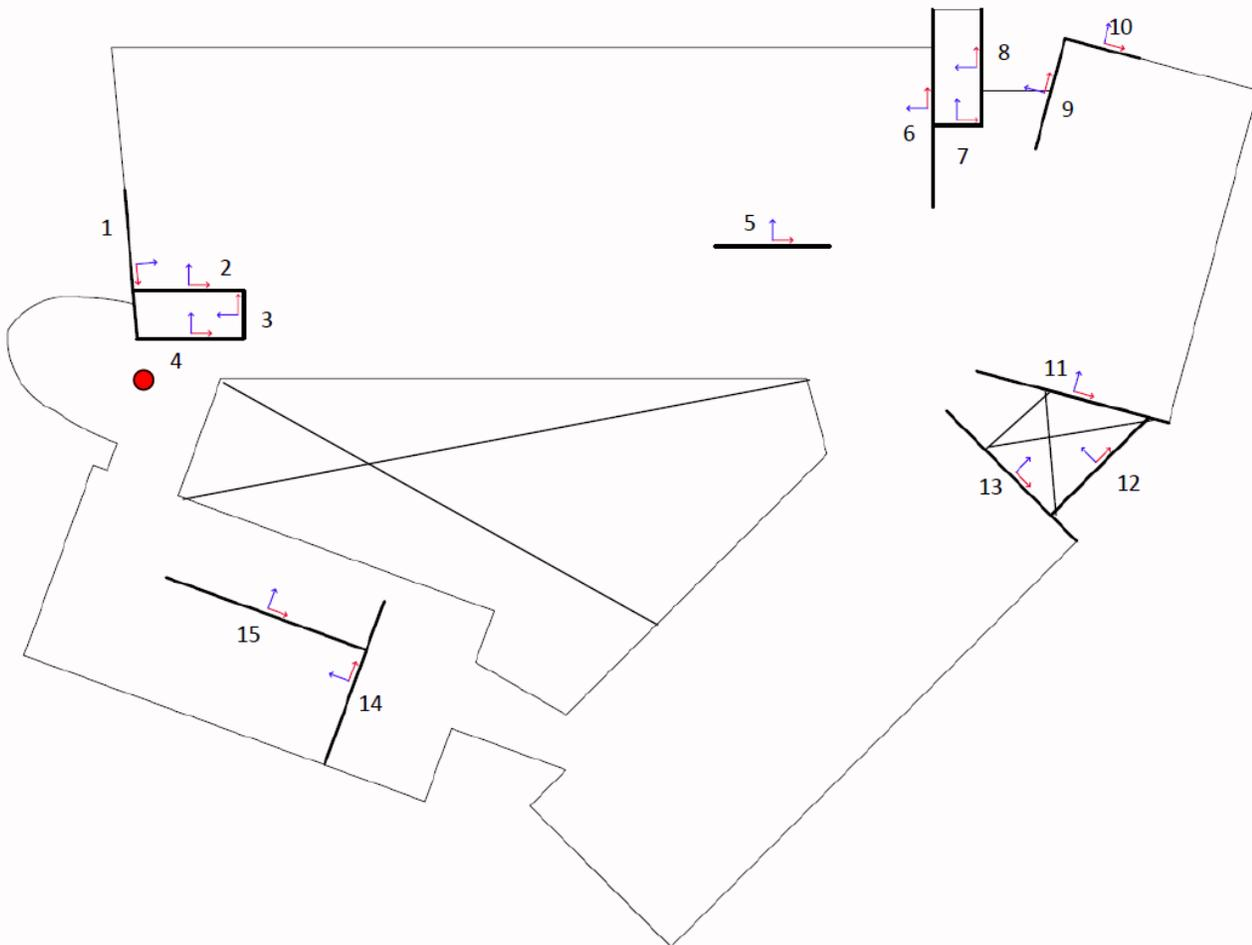
**Figure 23** Floor plan showing shear wall pier labels and axes used to obtain shear results. The red axis corresponds to ETABS’ “V2” (strong) axis, and the blue axis corresponds to ETABS’ “V3” (weak) axis. Red dot is considered (0,0) ft location.
