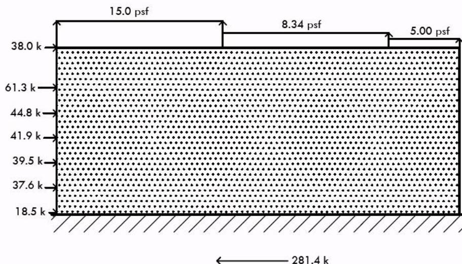
Figure 13 List and diagram of N-S direction wind forces.
