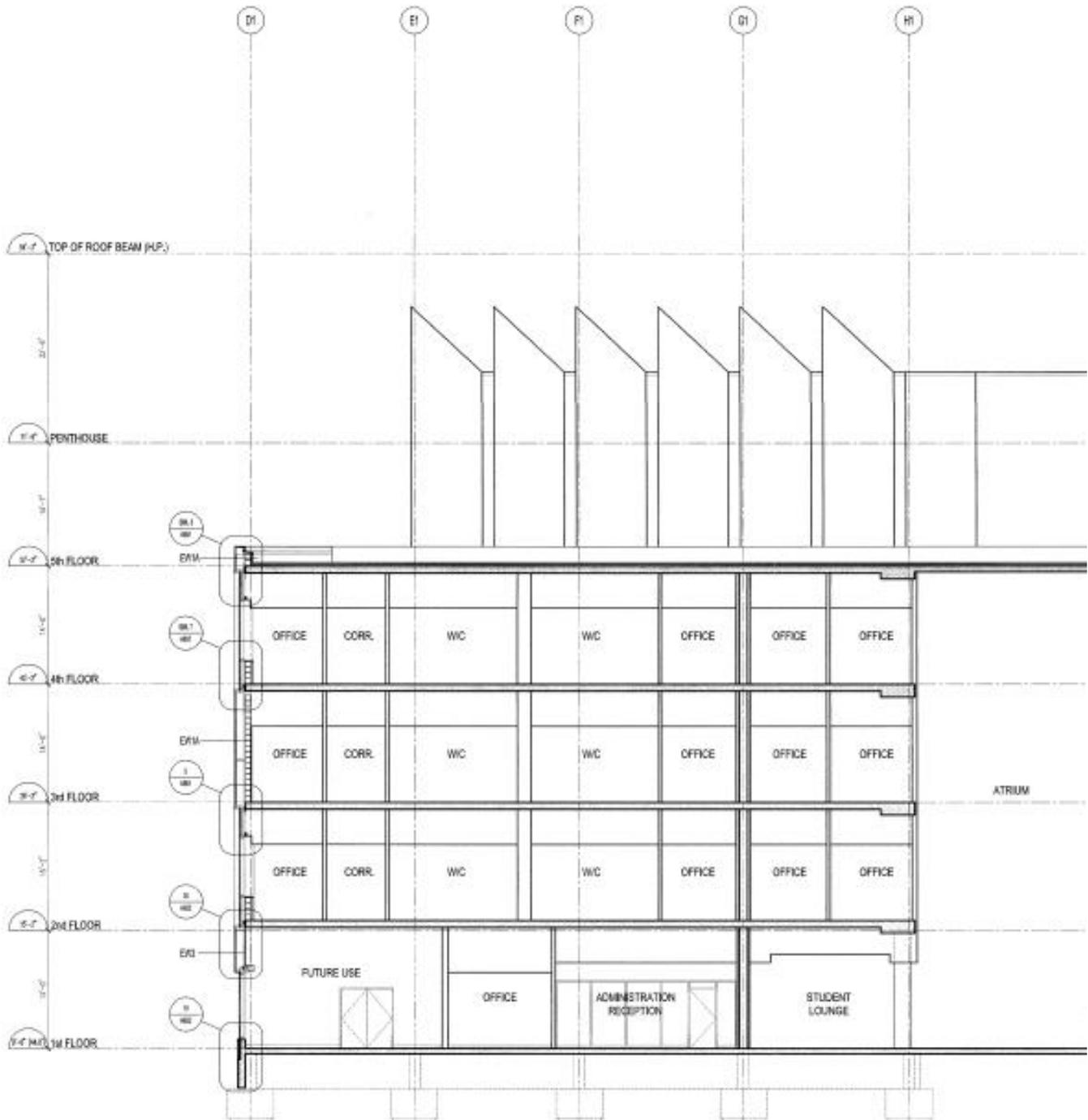
Figure D.5 Section 4 through portion of building at -20° rotation (see Figure 1), taken from 3/A403.
