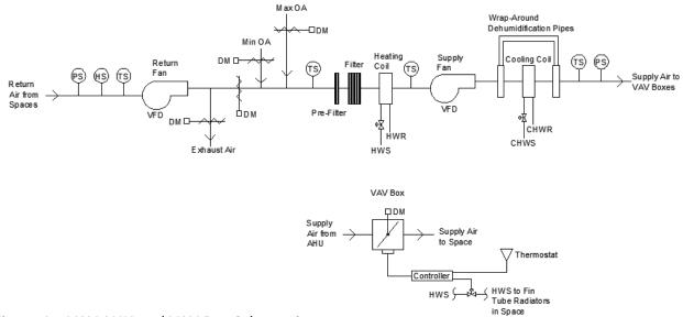
Figure 1 – VAV AHU and VAV Box Schematic
