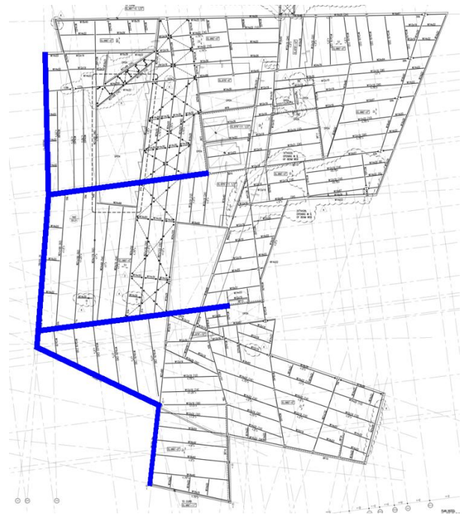
Figure 5. Highlighted truss elements from Building 1 Level 8.
