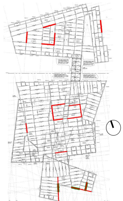
Figure 6. Level 6 Braced Frames and Shear walls
