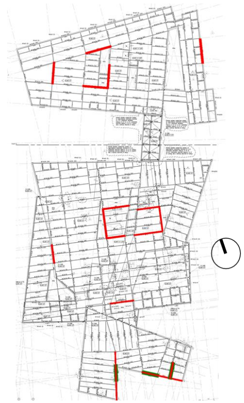
Figure 10 – Braced Frames and Shear Wall Locations floor framing plan.
