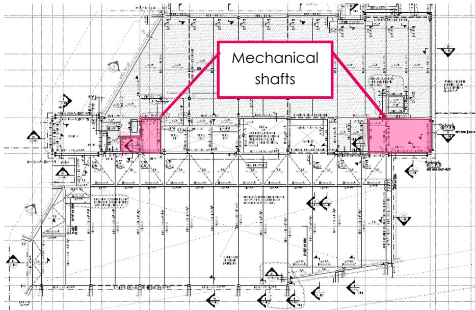
Figure 5 The location of mechanical shaft on 9<sup>th</sup> floor (S-109)
