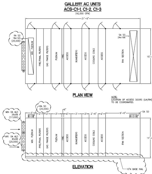
Figure 4 Dimension of a typical air conditioning system in AAM
