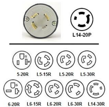
Figure 66 NEMA L14-20R Diagram, google.com
