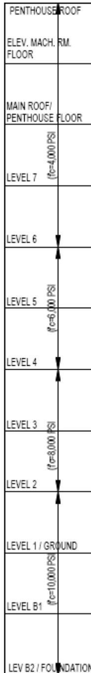
Figure 6: Variations in column concrete strengths per level
