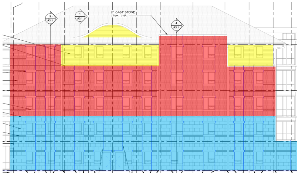
Figure 26 Façade Types, South Elevation – South Wing – Building C Details from Sheet A2.1C - Architectural Plans – WTW
