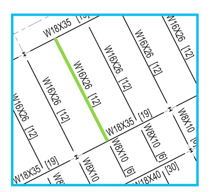
Typical Composite Beam Design (1<sup>st</sup>/2<sup>nd</sup>/3<sup>rd</sup> Floor Small Classroom)
