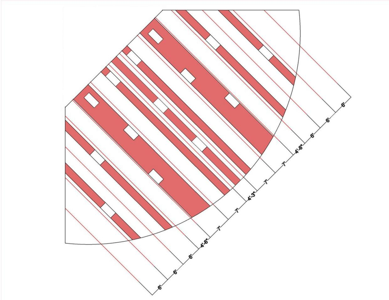
In the figure above, the skylight spans are highlighted in red to show where the structural joist cannot be placed. Only in the white parts could the joists span the whole length of the auditorium. Slight adjustments were needed to the placement of the skylights in order to accommodate the spans between joists. A span of 7' was chosen to be the largest span acceptable. This decision was based on the upper limitations of LH joists with they're depth and self-weight restrictions.
