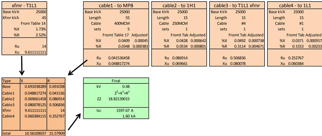
So the final  $I_{sc}$  for this circuit that ends with panelboard 1L1 comes to 1,598 Amps of fault-current.
