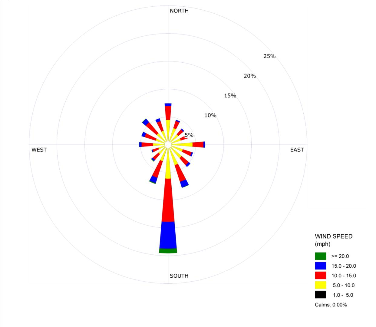
This wind rose shows that wind is mostly from the south. In order for the disks to spin, there needs to be east or west direction wind. By this wind rose, you can see that wind comes from the East 22% of the time, and from the West, also about 22% of the time. So totally, the solar disks should be able to be spinning about 44% of the day. This means they could spin up to 10.5 hours out of the day. The wind rose also shows that the average wind speed is about 10 mph.
