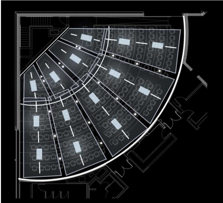
The pictures above illustrate the new ceiling design for the auditorium. The original ceiling, made of GWB, slopes up in the front of the room, levels off in the middle and then slopes back toward the back of the room. The new ceiling is laid out in a radial fan pattern. It is made up of nine panels of
