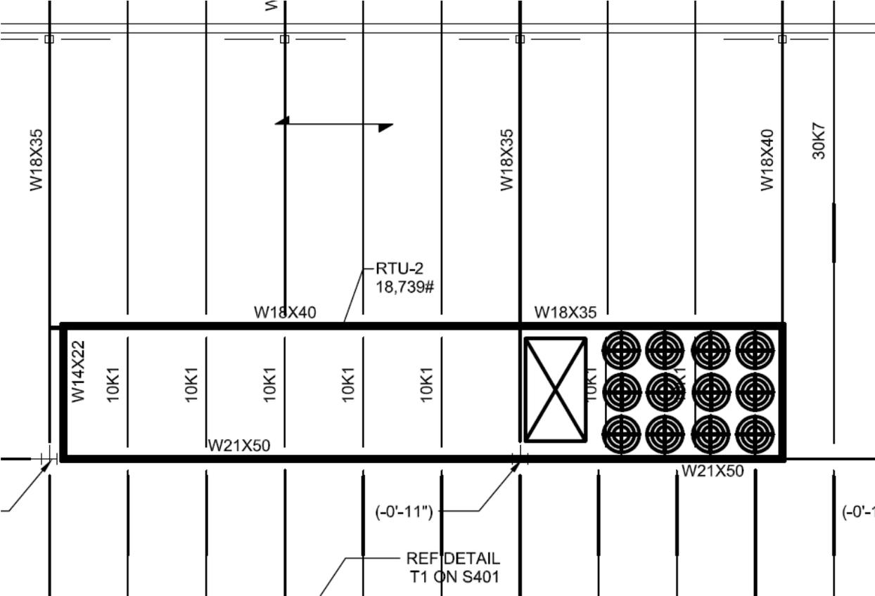
Figure E.2: Joist Calculation for Column Lines 2-4 (typical)
