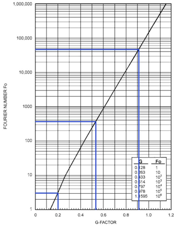
**Fig. 15 Fourier/G-Factor Graph for Ground Thermal Resistance**
