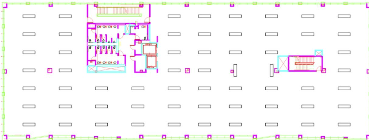
Figure 12: Sample Layout of Active Chilled Beams in 201 Rouse Office Space
