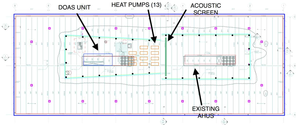
The first major change to the roof load was the removal of AHU #2 and the acoustical screen on the east side of the building. The removal of these components required the reanalysis of the supportive beams and joists; see Figures E.2 and E.3 for the structural calculations. This analysis
