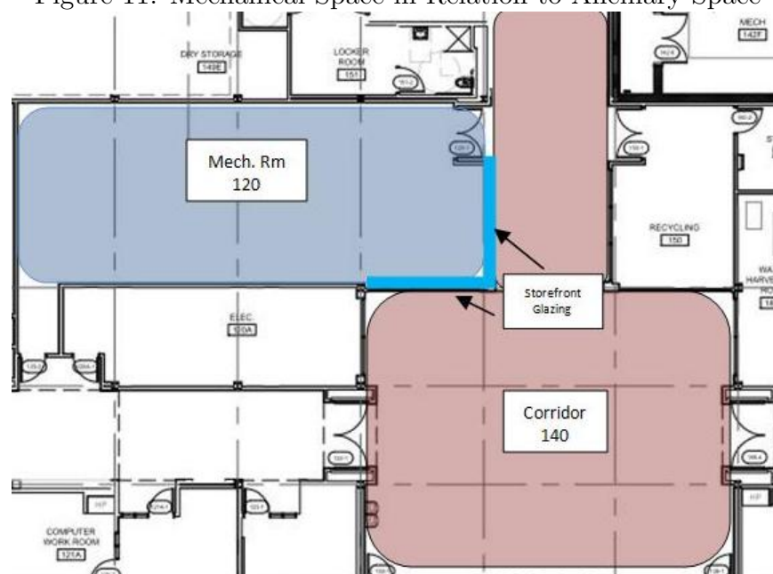
Figure 11: Mechanical Space in Relation to Ancillary Space
