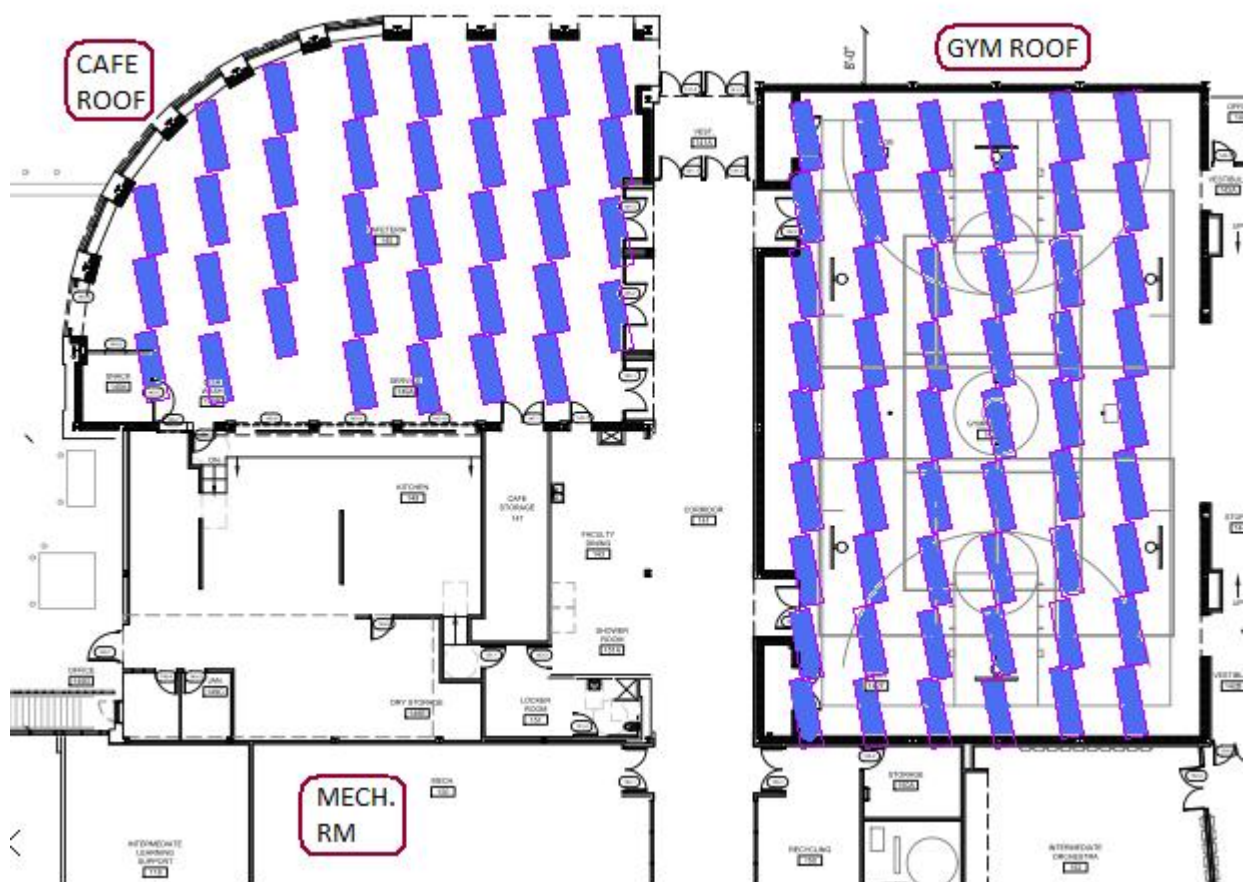
Figure 10: Placement of Solar Array on Cafe and Gym Roofs
