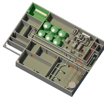
Figure 13. Anaerobic digestion plant located in building mechanical room.
