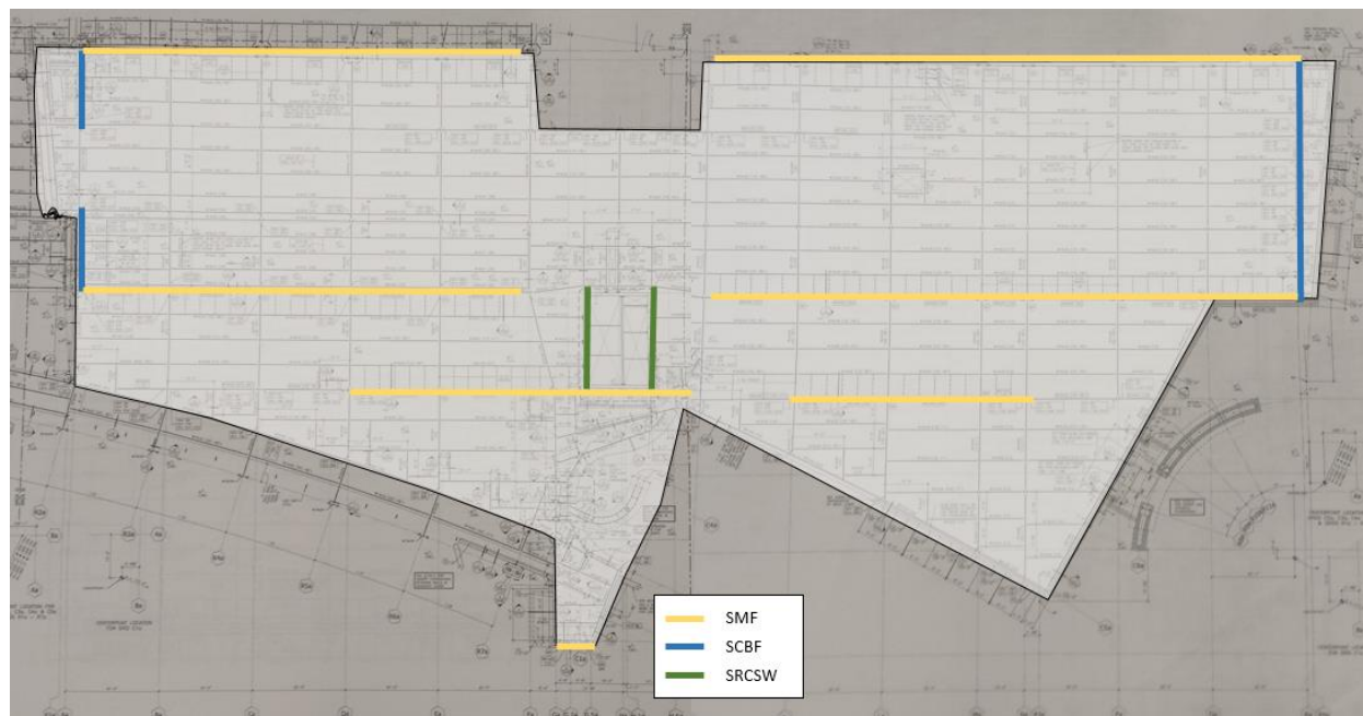
Figure 10: LFRS element location in bed tower
