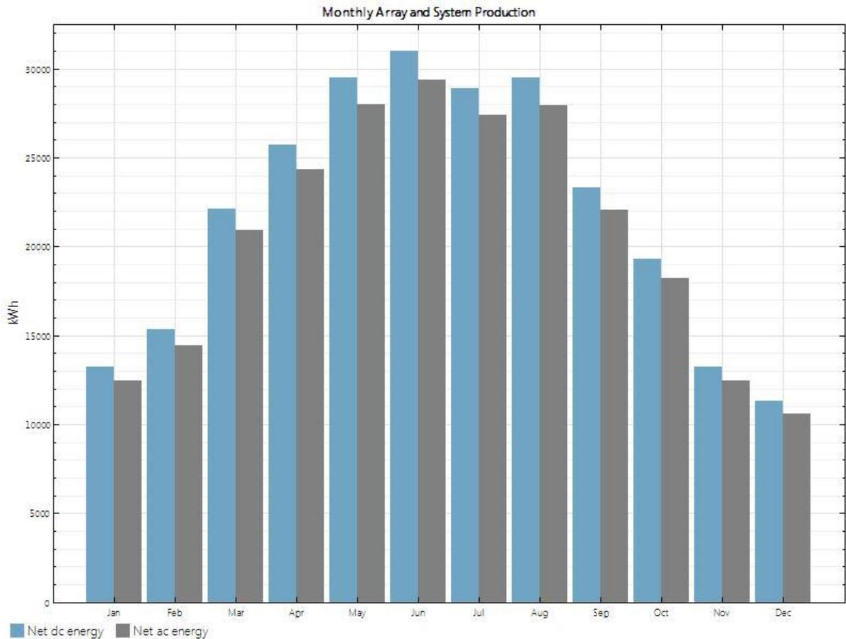
Figure 66 | DC vs. AC Energy Production | SAM
