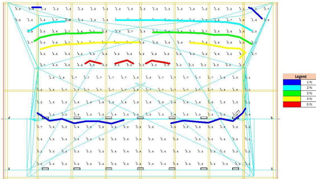
Figure 27 | Light Box Contour Plot | AGi32
