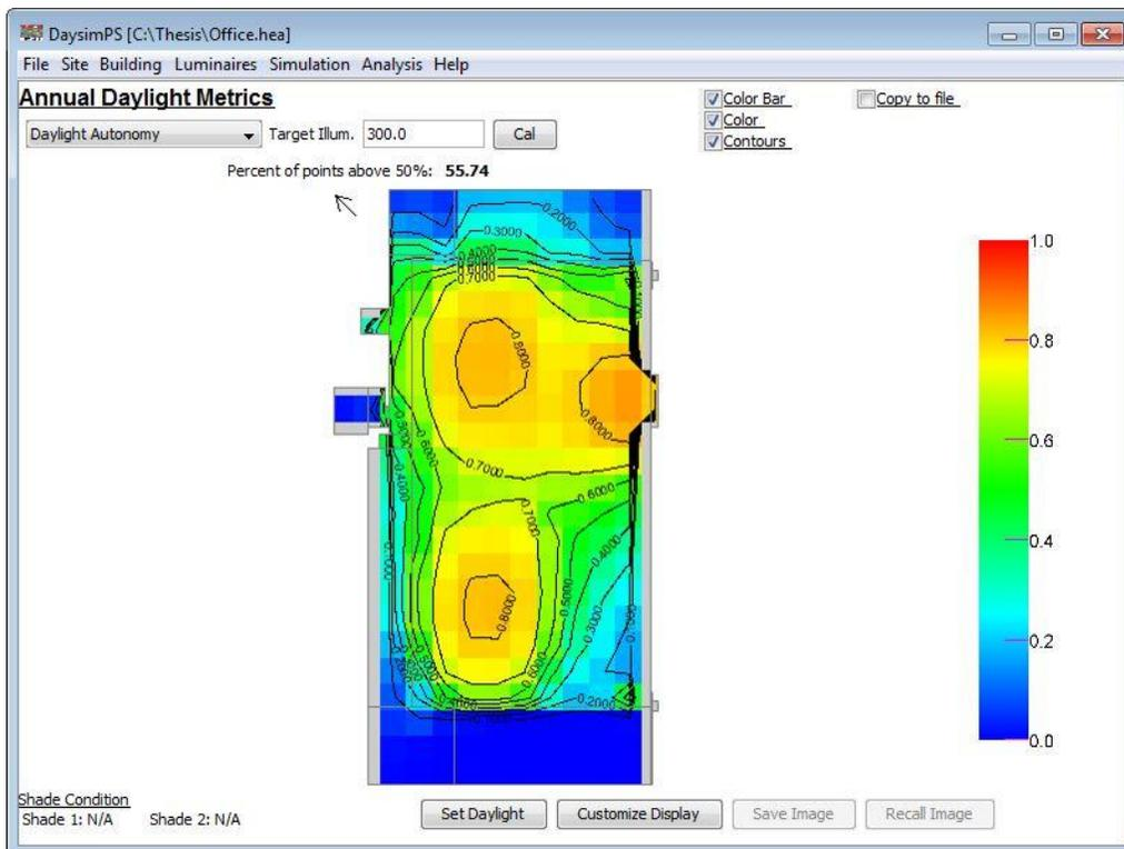
Figure 76 | Daylight Autonomy | Daysim
