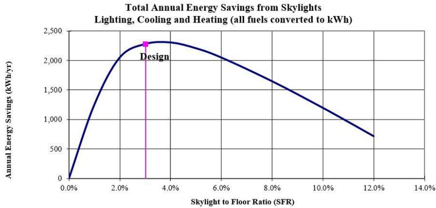
Figure 79 | Annual Energy Savings vs. Skylight to Floor Ratio | SkyCalc
