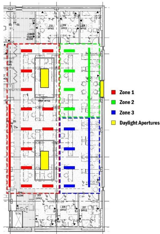
Figure 72 | Office Lighting Daylight Zones
