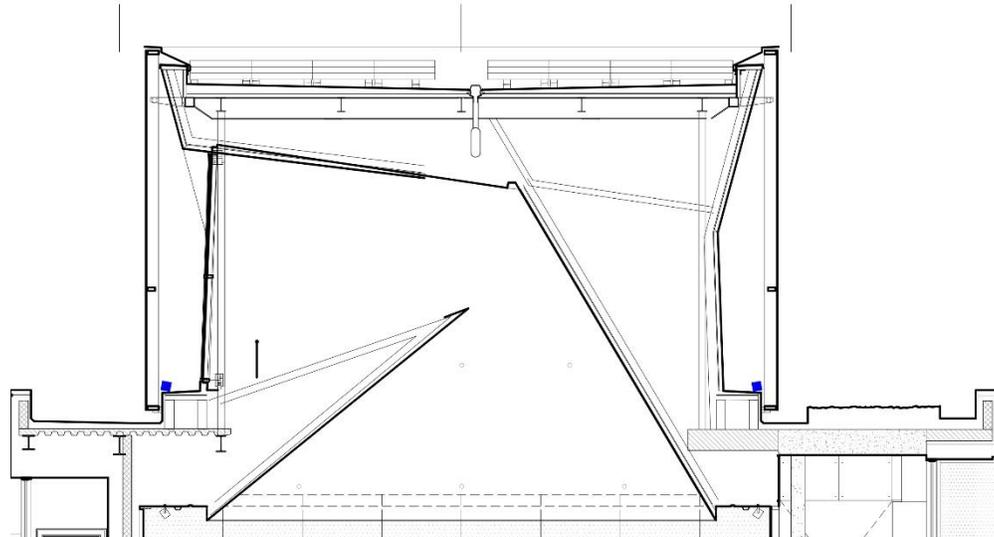
Figure 22 | Light Box Section
