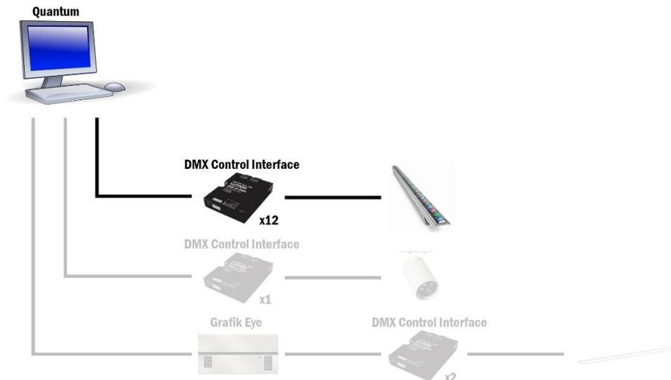
Figure 23 | Light Box Control Diagram
