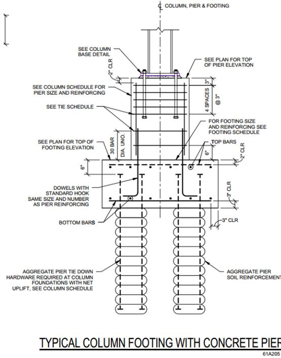
FIGURE 2- TYPICAL COLUMN FOOTING WITH CONCRETE PIER
